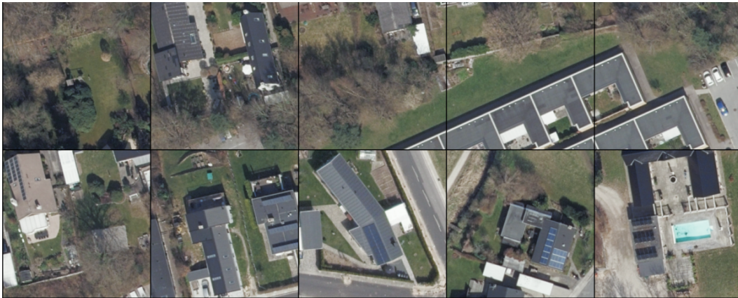
Figure 1: Illustrations of images from Herlev municipality (test set). Top row without PV, bottom row with PV.
