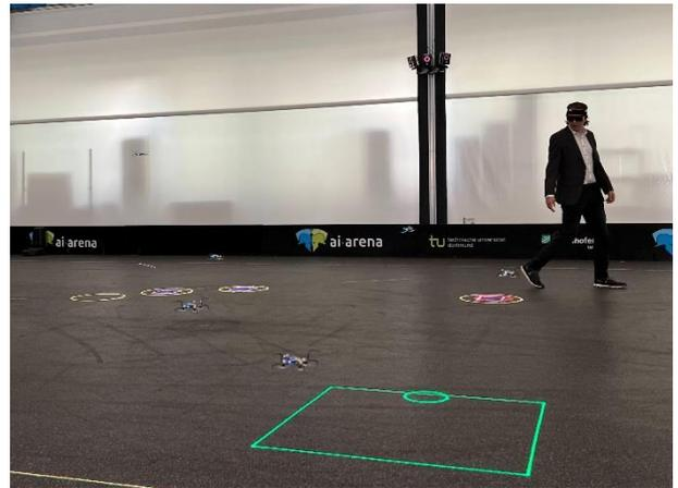
**Figure 6. Experimental setup showing UAVs in wander mode performing the transportation task alongside humans in the test area.**
