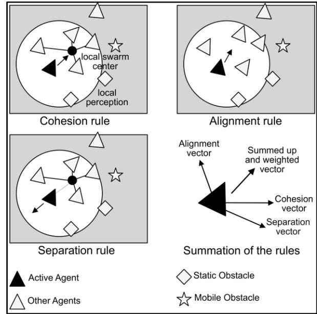
**Figure 3. Schematic representation of the three basic rules for simulated swarm behavior [21]. Mobile obstacles are people moving with headgear, and static obstacles could be the charging station, walls, or shelves.**
