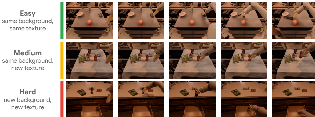
Figure 10: “Backgrounds” evaluations focus on testing the performance of RT-1 on settings with different table textures and different backgrounds, such as those found in kitchens never trained on. These visual differences are quite pronounced, which in the most challenging case entails a new kitchen with different counter texture, different lighting conditions, different counter material, and a different background.
