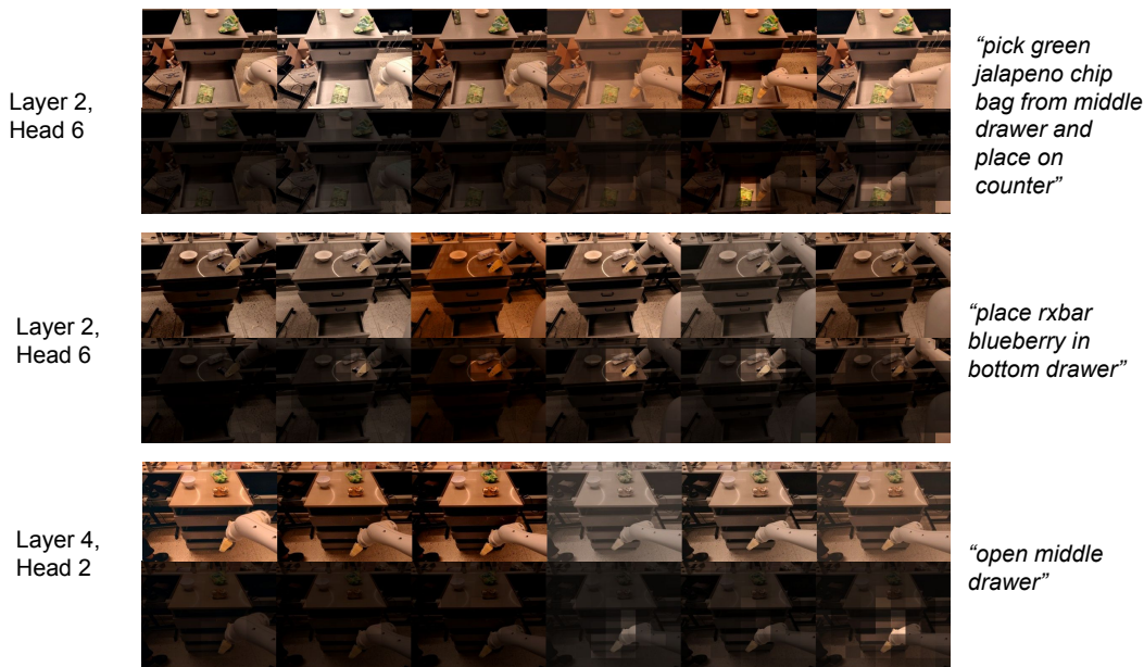
Figure 13: In this figure we show the attention map of the RT-1 policy. Different layers and heads generally focus on different part of the image. Most commonly, they focus on the parts of the scene with the richest interaction affordances, such as graspable objects. For example, Layer 2 Head 6 focuses on the jalapeno chips and pepsi can in grasping tasks; and Layer 4 Head 2 focuses on the drawer in drawer opening tasks.
