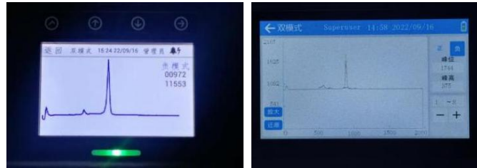
Figure 10. Measured detector responses: (a) original design; (b) new design.
