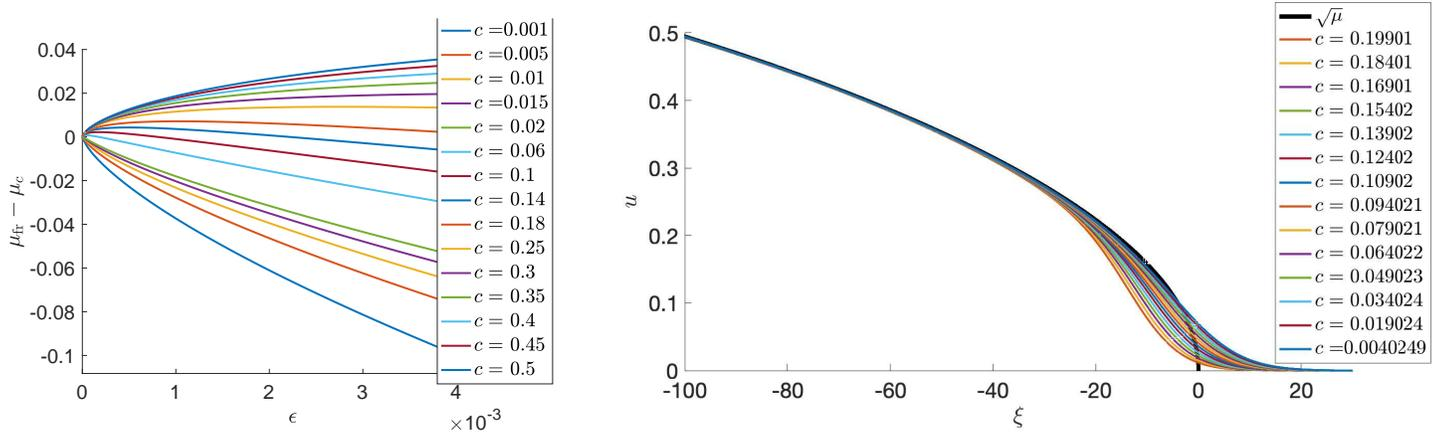
Figure 8.2: Left: plots of the numerically measured difference  $\mu_{\text{fr}} - \mu_c$  against  $\epsilon$ , for a range of  $c$  values (given in legend), curves increase as  $c$  increases; Right: Plots of the front profile near  $\mu = 0$  for a range of  $c$ -values (in legend), curves decrease as  $c$  increases with  $\epsilon = 0.0025$  fixed.
