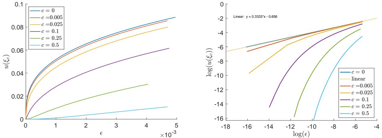
Figure 8.3: Left: plot of the values  $u(\xi_c)$  against  $\epsilon$  for a range of speeds  $c$ . Note the curves from convex to concave as  $c$  decreases; Right: Log-log plot of  $u(\xi_c)$  against  $\epsilon$ , showing that the front height becomes exponentially small in  $\epsilon$  for moderate speeds  $c$ . Also included is a linear fit of the  $c = 0$  curve (light yellow, with fit equation printed), indicating that  $u(\xi_c)$  scales like  $\epsilon^{1/3}$  in this case.
