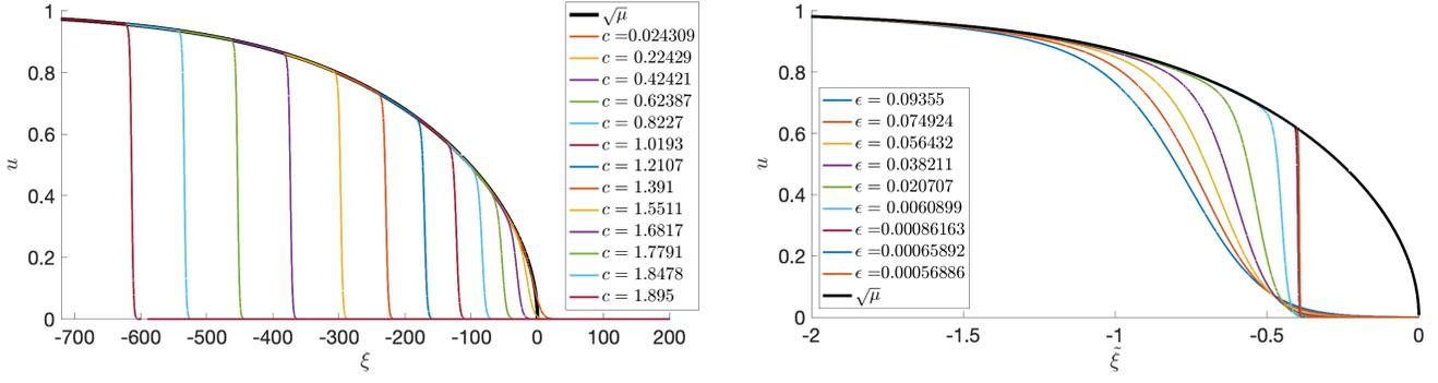
Figure 1.1: Results of numerical continuation of the traveling wave of (1.3)-(1.4) using AUTO07p. Left: Solutions  $u(\xi)$  for a range of  $c$ -values (values in legend) with  $\epsilon = 0.0025$  fixed. Right: Solutions  $u$  against the rescaled variable  $\tilde{\xi} = \epsilon\xi$  for a range of  $\epsilon$  values (values in legend) with  $c = 1.2$  fixed, along with  $\mu(\tilde{\xi})^{1/2}$  for  $\tilde{\xi} < 0$ .
