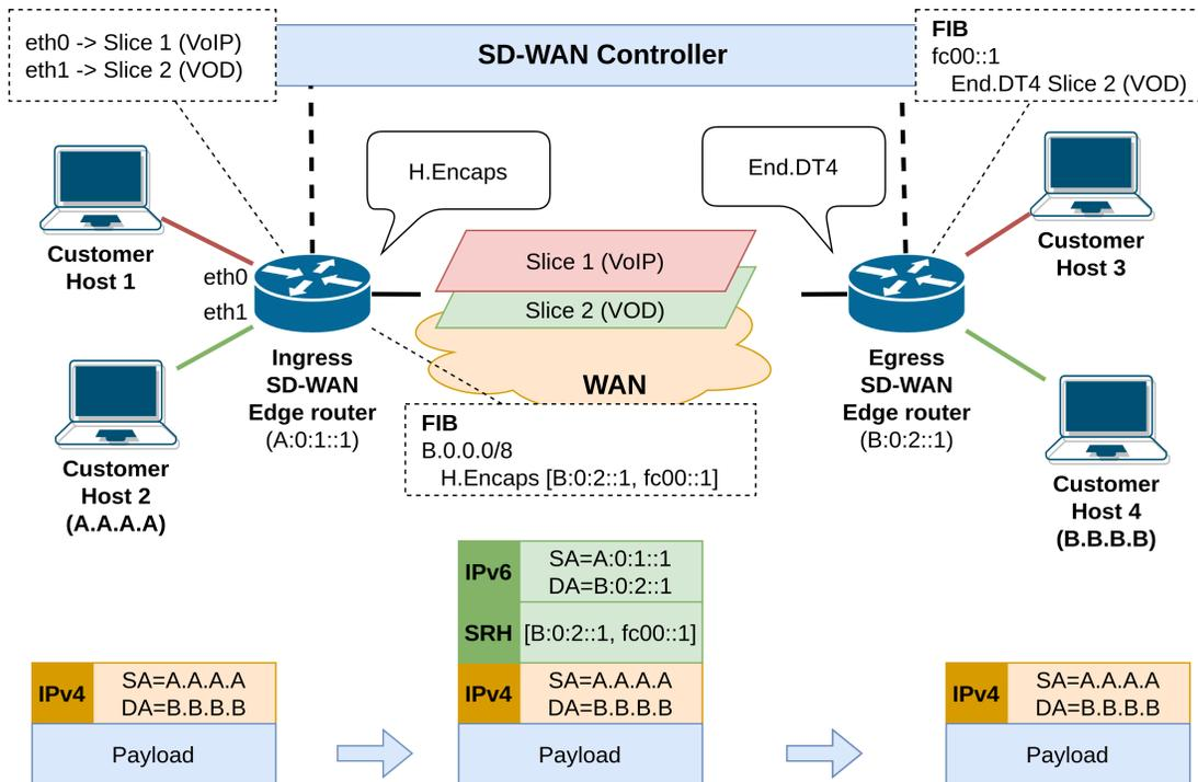
Fig. 4: SD-WAN Network Slicing scenario (SRv6).
