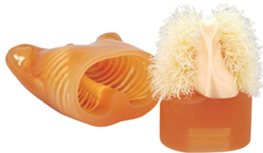
Figure 6: LUNGMAN phantom (Kyoto Kagaku Co. Ltd., Japan) was used for in-plane spatial resolution inspection.
