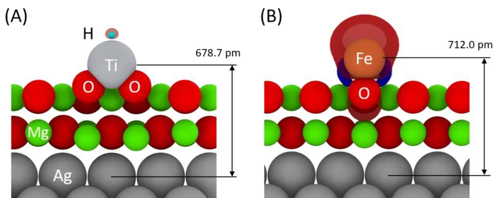
DFT-calculated geometries of Ti (A) and Fe (B) atoms adsorbed on 2ML-thick MgO on Ag(100).
