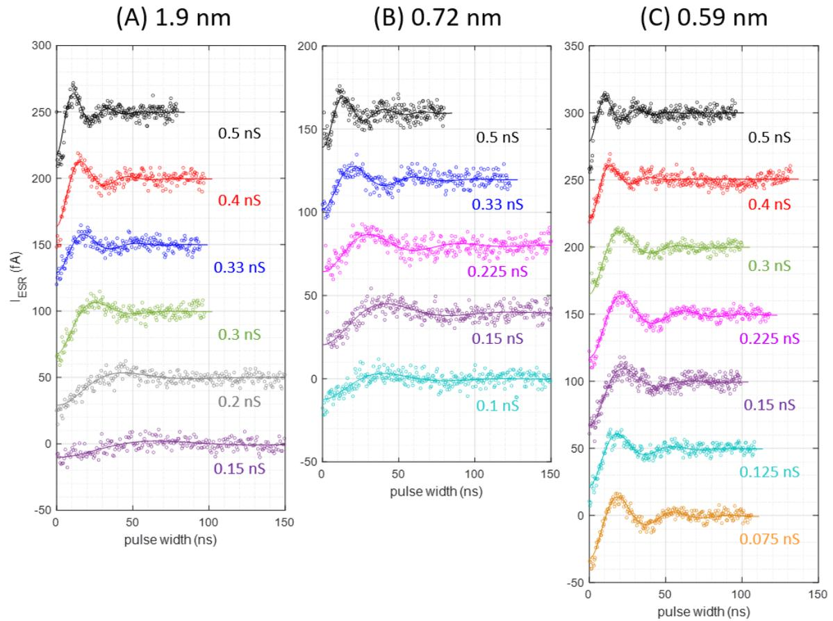
**Tunnel conductance dependence of Rabi oscillations measured on the Ti-Fe pairs shown in Figs. 1b-d.** Solid curves are the fits using an exponentially decaying sinusoidal function, resulting in the Rabi rates in Fig. 2c. ( $I_{\text{DC}} = 10$  pA,  $T = 1.2$  K,  $B_{\text{ext}} = 0.9$  T,  $\theta_{\text{ext}} = 82^\circ$ ).
