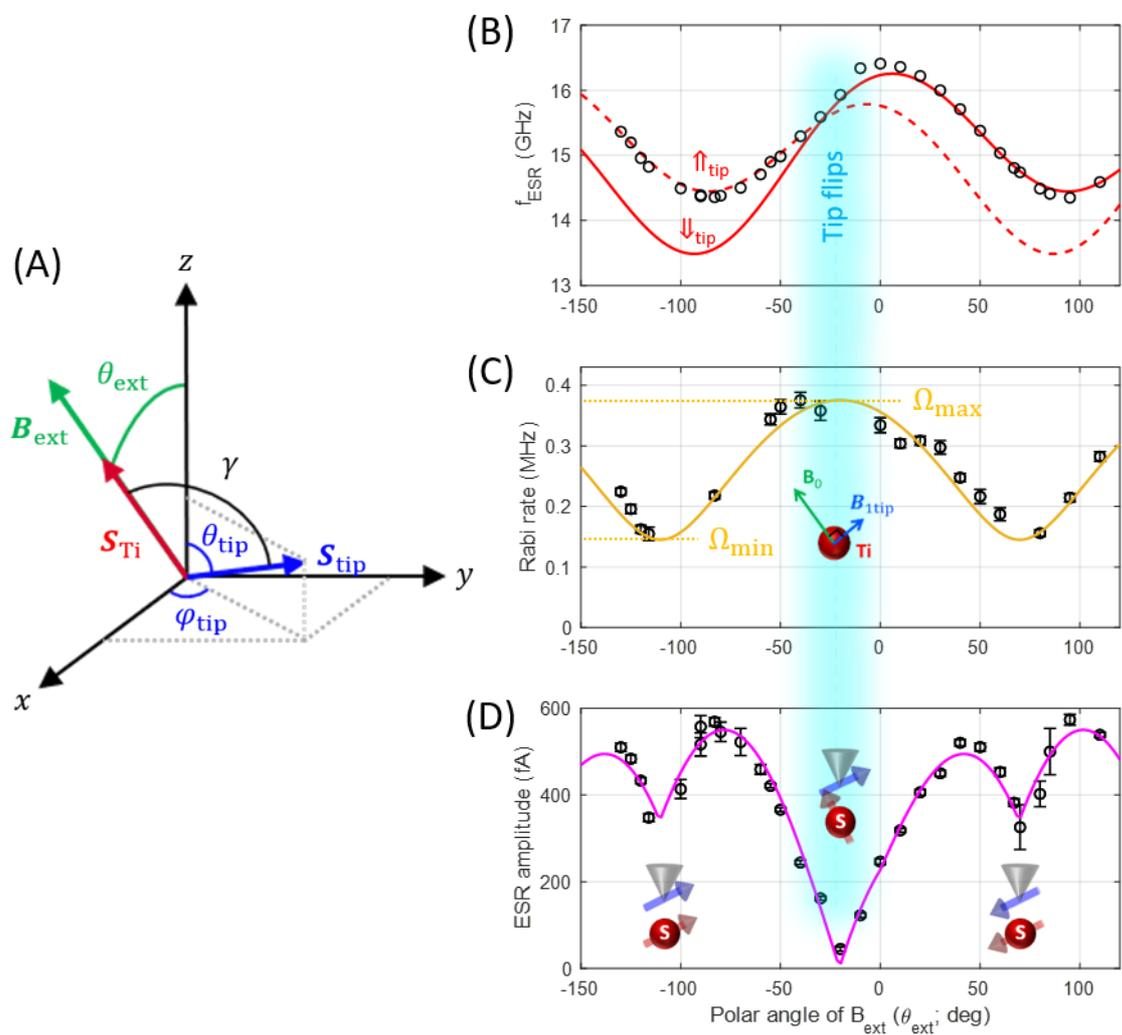
**Analysis of data from an isolated Ti spin.** (A) A schematic showing the definitions of the angles used in the model. Plots of (B) ESR frequencies, (C) Rabi rates, and (D) ESR amplitudes measured from an isolated Ti spin as a function of the polar angle of the external field ( $\theta_{\text{ext}}$ ) ( $I_{\text{tunn}} = 10$  pA,  $V_{\text{DC}} = 30$  mV). Solid curves are the fits using the model discussed in the text.
