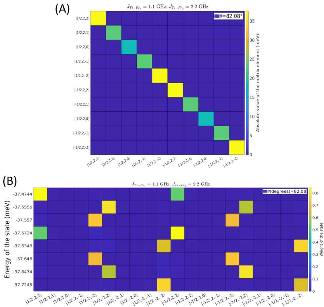
**Model Hamiltonian of a Fe-Ti-Fe spin complex.** Checkerboard representations of (A) subset of the Hamiltonian matrix for the first Fe ( $\text{Fe}_1$ ) is up ( $\uparrow$ ;  $m_{\text{Fe}_1} = 2$ ) and (B) the eigenstates of the eight lowest energies. The spin states are labelled according to the array of three spins,  $|m_{\text{Ti}}, m_{\text{Fe}_1}, m_{\text{Fe}_2}\rangle$  ( $B_{\text{ext}} = 0.9 \text{ T}$ ,  $\theta_{\text{ext}} = 82^\circ$ ).
