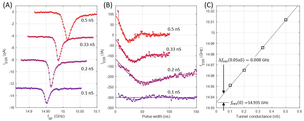
**Tunnel conductance dependence of CW- and pulsed-ESR on an isolated Ti.** (A) CW-ESR spectra and (B) Rabi oscillations measured on the same tip and Ti atom as used for the data in Fig. S13. (C) ESR resonance frequencies extracted from the spectra in (A). Solid line is a linear fit. ( $I_{\text{DC}} = 10$  pA,  $T = 0.4$  K,  $B_{\text{ext}} = 0.6$  T,  $\theta_{\text{ext}} = 72^\circ$ ).
