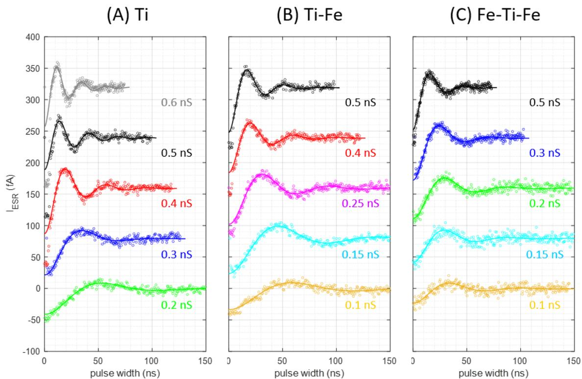
**Tunnel conductance dependence of Rabi oscillations measured on the Fe-Ti-Fe complex shown in Fig. 5.** Solid curves are the fits using an exponentially decaying sinusoidal function, giving the Rabi rates  $\Omega$  shown in Fig. 5c. ( $I_{\text{DC}} = 10$  pA,  $T = 0.6$  K,  $B_{\text{ext}} = 0.9$  T,  $\theta_{\text{ext}} = 82^\circ$ ).
