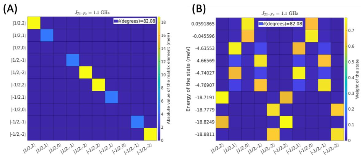
**Model Hamiltonian and eigenstates of a Ti-Fe pair.** Checkerboard representations of (A) the Hamiltonian Eqn. S2 for a pair of Ti-Fe separation of 0.72 nm and (B) its eigenstates ( $B_{\text{ext}} = 0.9 \text{ T}$ ,  $\theta_{\text{ext}} = 82^\circ$ ).
