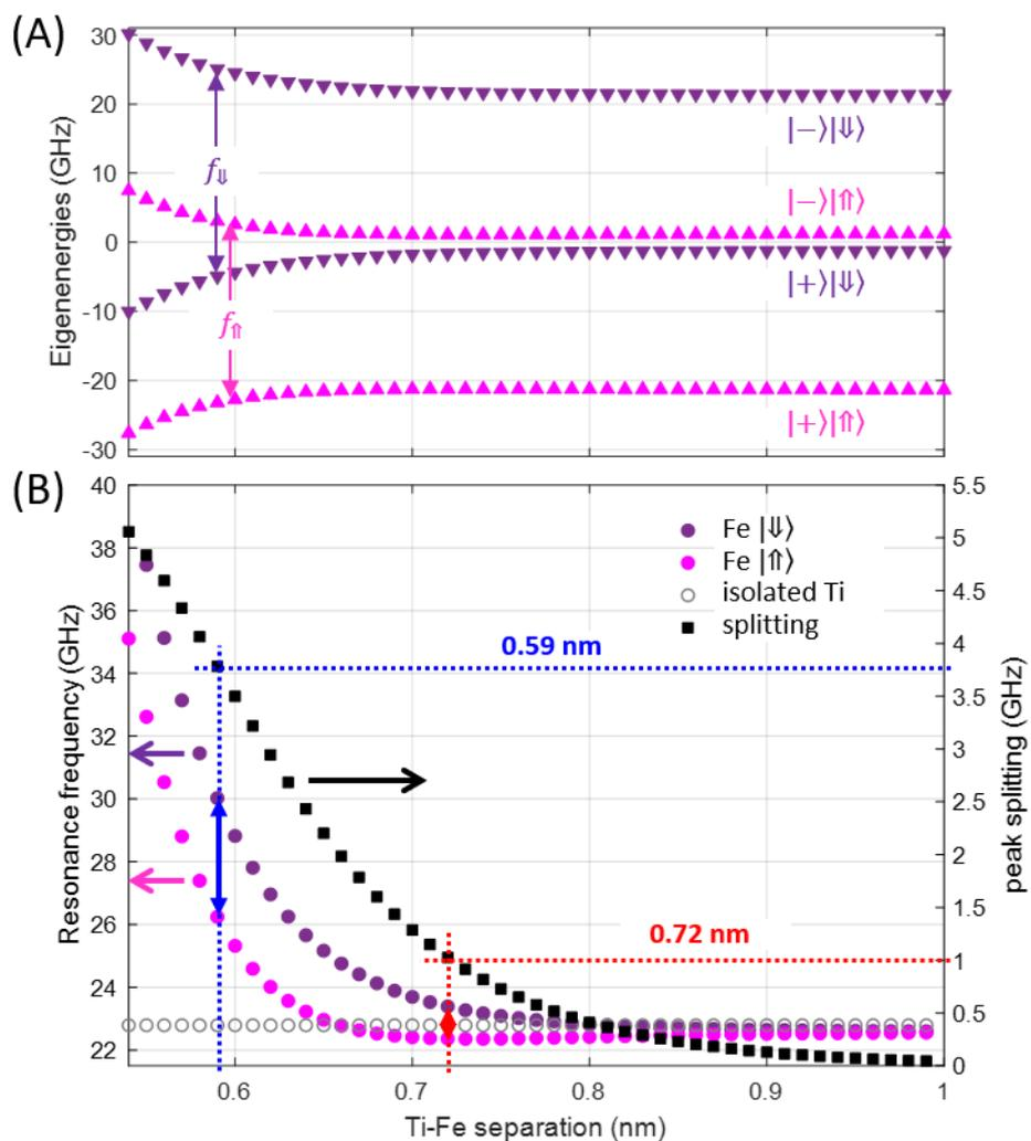
**Model simulations of ESR transitions of Ti in a Ti-Fe pair.** (A) Eigenstates and (B) peak splitting as a function of Ti-Fe separation using the model Hamiltonian  $\hat{H}_{\text{pair}}$  (Eqn. S2). The dependence of  $J_{\text{Ti,Fe}}$  on the Ti-Fe separation (Fig. S1B) was used. In (A), we shifted the four as-calculated eigenenergies by adding the Zeeman energies of the Fe spin for the two ESR transitions ( $f_{\uparrow}$  and  $f_{\downarrow}$ ) to be clearly visible.
