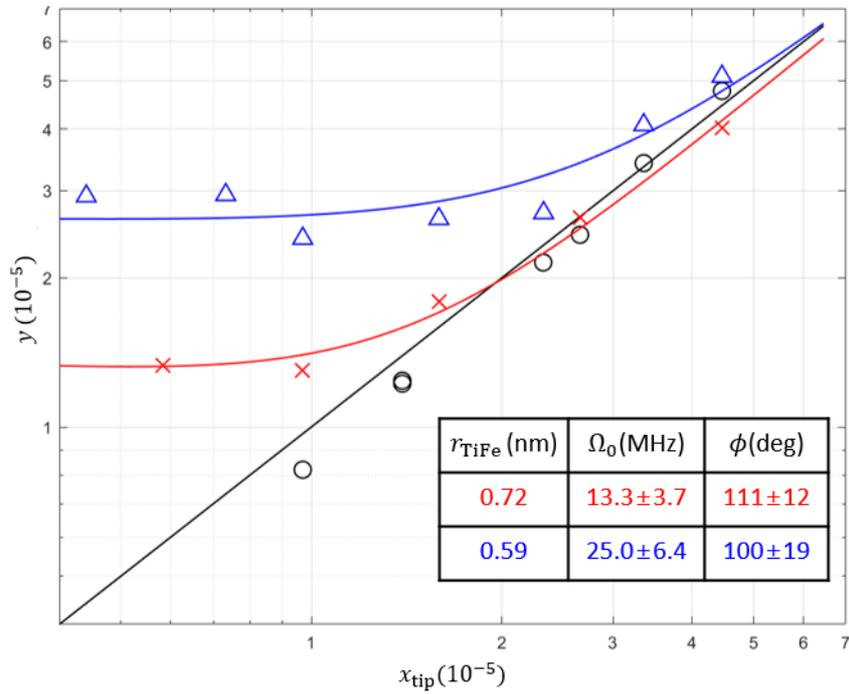
**Fits of Rabi rates vs. tunnel conductance for the three cases in Fig. 2C.** Replot the data in Fig. 2C using the model discussed in the above text with the x- and y-axis variables defined in equations (S10) and (S11). The fits resulted in the parameters  $\Omega_0$  and  $\phi_{\uparrow}$ , as shown in the inset.
