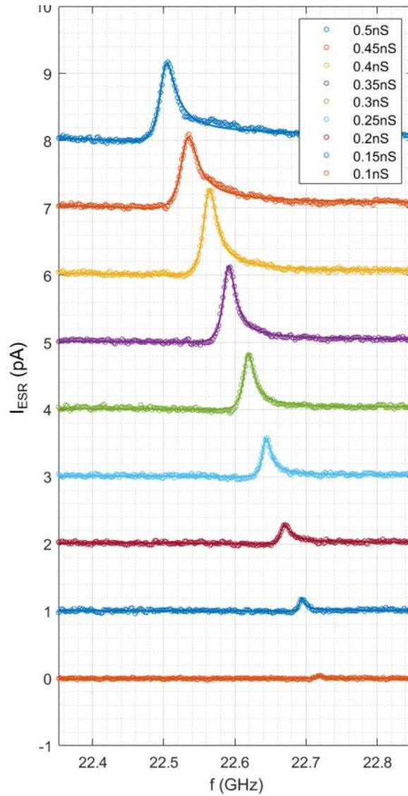
**Tunnel conductance dependence of ESR spectra of a single Ti measured with the same tip used in Fig. 3.** As the tip was retracted from the Ti spin, the peak height monotonically decreases, and it vanishes. ( $V_{\text{DC}} = 50$  mV,  $T = 1.2$  K,  $B_{\text{ext}} = 0.9$  T,  $\theta_{\text{ext}} = 82^\circ$ ).
