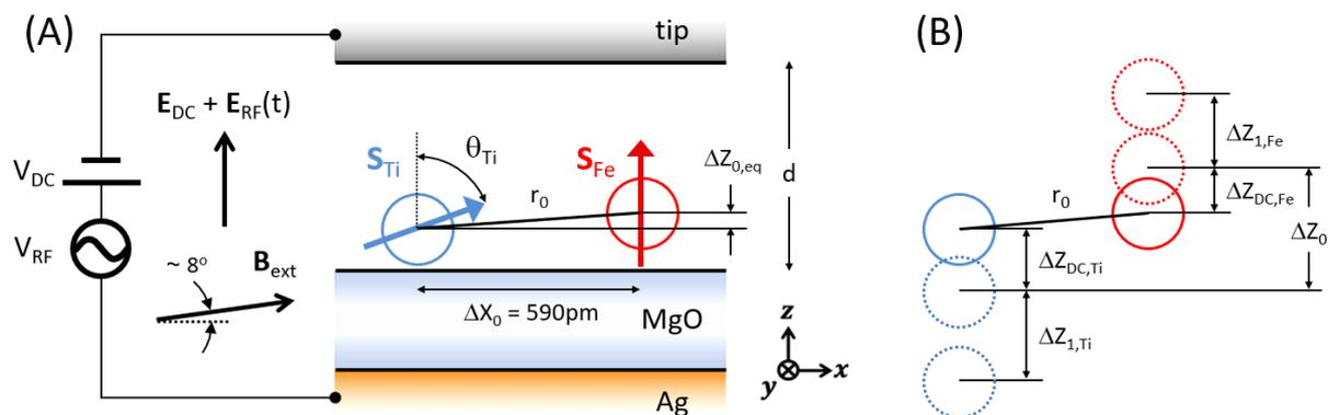
**Schematic of a Ti-Fe pair in the tunnel junction to derive piezoelectric motions of the spins.**
