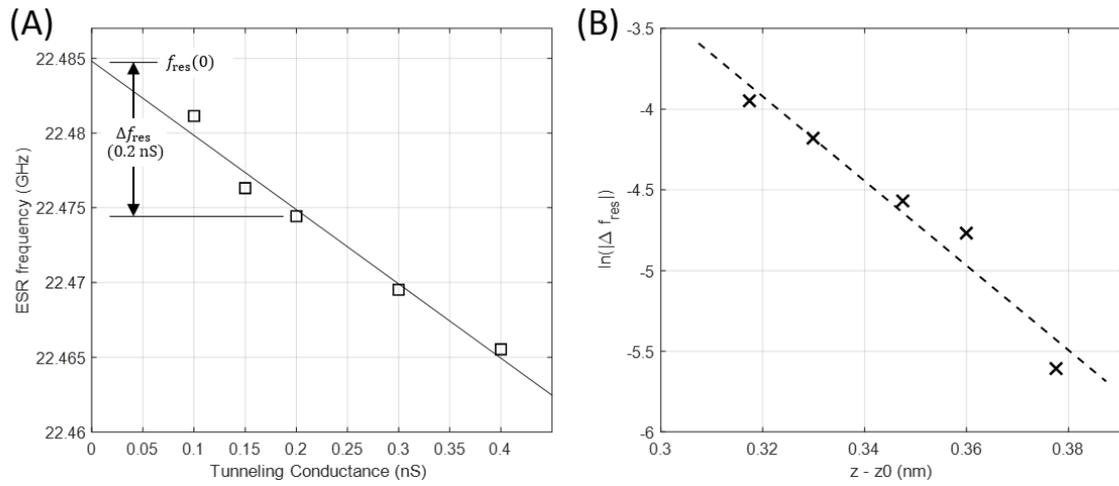
**ESR resonance frequency on an isolated Ti. (A)** Resonance frequency ( $f_{res}$ ) as function of tunnel conductance. **(B)** Shift of  $f_{res}$  ( $\Delta f_{res}$ ) measured from the  $f_{res}$  at zero conductance, as indicated in (A), as a function of tip height ( $z$ ). Using as-obtained  $d_0$  and  $\sigma_0$  in the discussion above, we converted the measurement tunnel conductance into the tip height ( $z$ ). The solid lines are the linear fits of the plots.
