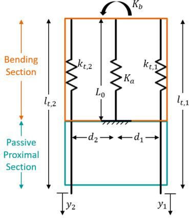
Fig. 5: Planar spring model for two tendons:  $L_0$ ,  $K_a$ , and  $K_b$  are the length, axial stiffness, and bending stiffness of the articulation section;  $l_{t,i}$ ,  $k_{t,i}$ ,  $d_i$ , and  $y_i$  are the undeformed length, stiffness, distance from the central axis, and displacement of tendon  $i$ .
