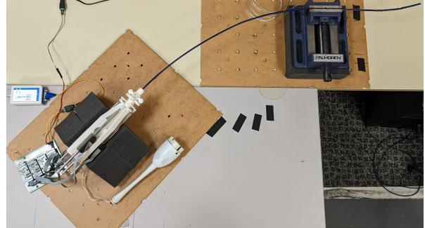
(b) passive proximal section bent to 45° angle
