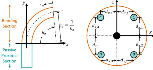
Fig. 4: Conceptual side-view and cross-section.  $\theta_z$ ,  $\kappa_z$ , and  $r_z$  are the bending angle, curvature, and radius of curvature about the  $z$ -axis (in the  $xy$ -plane).  $(d_{xi}, d_{zi})$  are the coordinates of tendon  $i$  relative to the central axis ( $y$ -axis) of the robot.
