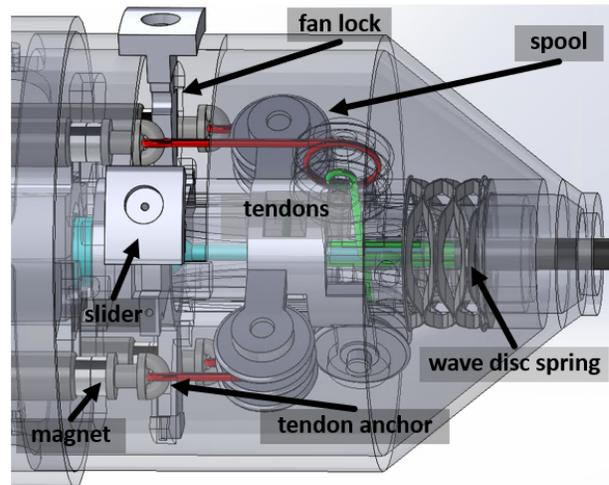
Fig. 2: Disposable portion of the robot.
