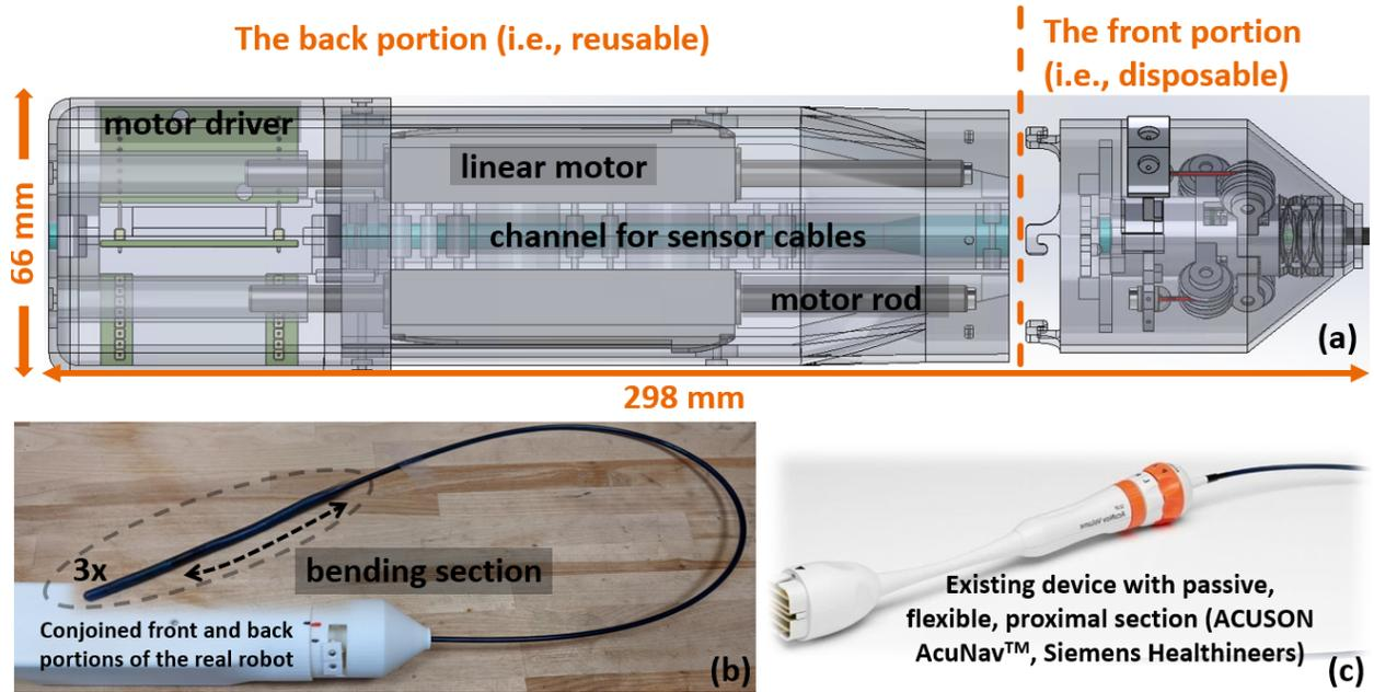
Fig. 1: An overview of the catheter robot.
