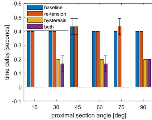
Fig. 13: Bending angle time delay for different compensation types and proximal section angles (xy-plane input).
