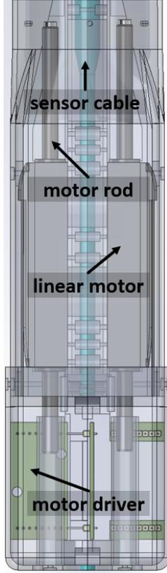
Fig. 3: Reusable portion of the robot.
