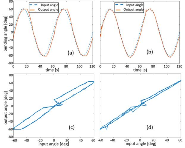
Fig. 9: One result for yz-plane bending: (a) Time vs output angle without compensation (b) Time vs output angle with hysteresis compensation (c)(d) The input angle vs the output angle without/with hysteresis compensation.
