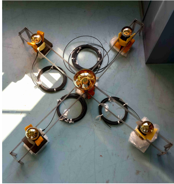
Figure 10: PMT holder: holding test.
