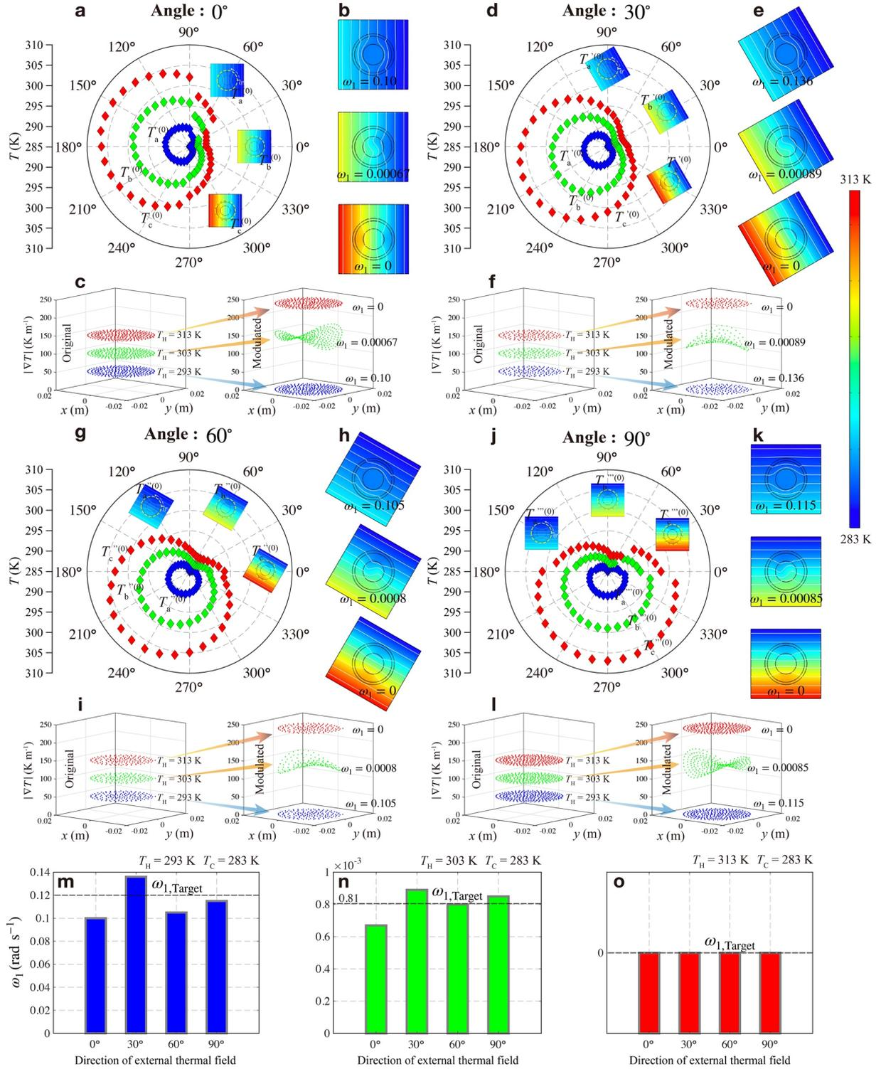
**Figure 2.** Response of the heat-enhanced thermal diffusion metamaterial in simulations. a)  $N = 36$  equally spaced temperature data  $T_a^{(0)}$ ,  $T_b^{(0)}$ ,  $T_c^{(0)}$  in the yellow dashed circle in static bilayer structures. The hot source is set as 293, 303, 313 K, respectively. The cold source is fixed at 283 K. The first data is the temperature of the position marked  $0^\circ$ . Each temperature
