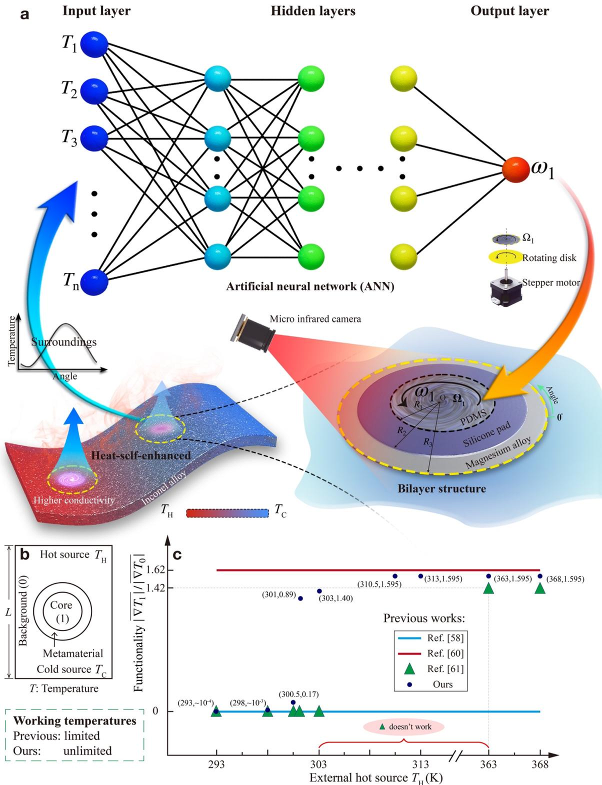
**Figure 1.** Architecture. a) Schematic of a deep learning-assisted active metamaterial. It comprises a micro infrared camera, a pre-trained artificial neural network, a stepper motor, and a bilayer structure. The infrared camera measures the temperature data ( $T_1, T_2, T_3, \dots, T_n$ ) of the bilayer structure's surroundings. Here, the bilayer structure consists of the inner layer (Silicone pad) and the outer layer (Magnesium alloy). The measured temperature data is input into the
