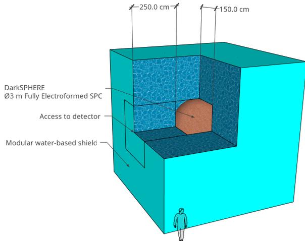
Fig. 9. Schematic representation of the conceptual shielding design used to estimate background rates for DARKSPHERE. The  $\text{Ø}3$  m electroformed-copper sphere is surrounded by a 2.5 m water shield and will be housed in the Large Experimental Cavern (LEC) at the Boulby Underground Laboratory.
