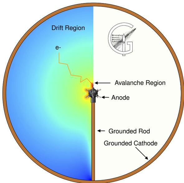
Fig. 1. Schematic and principle of operation of the spherical proportional counter. Particle interactions within the gas produce ionisation electrons, which drift towards the anode at the centre of the sphere. The anode shown is part of an 11-anode, multi-anode read-out system, ACHINOS. DARKSPHERE will operate with a multi-anode ACHINOS read-out sensor with 60-anodes. The copper used for the grounded cathode and grounded rod will be electroformed underground to minimise the background rate.
