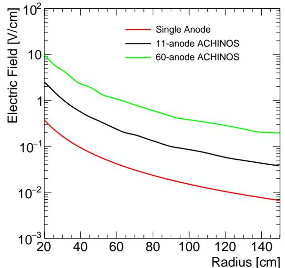
Fig. 3. Electric field magnitude in the drift-region as a function of radius for different read-out configurations in DARKSPHERE. Each ACHINOS read-out uses  $\varnothing 1$  mm anodes at the same voltage, and  $r_s = 10$  cm. Increasing the number of anodes increases the drift-region electric field magnitude without increasing the anode voltage.
