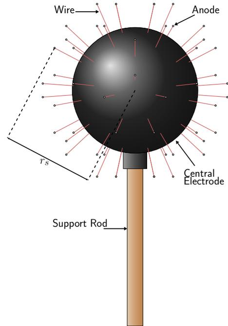
Fig. 5. Schematic of an 60-anode ACHINOS where the anodes are located at the vertices of a truncated icosahedron. The distance between each anode and the centre is labelled as  $r_s$ . The multi-anode ACHINOS enables the operation of larger and higher pressure spherical proportional counters by decoupling the drift-region electric field from the avalanche electric field.
