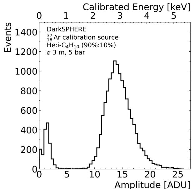
Fig. 8. Simulated energy spectrum recorded by DARKSPHERE equipped with a 60-anode ACHINOS, with  $r_s = 30$  cm, when an  ${}^{37}\text{Ar}$  gaseous calibration source is placed inside the detector. The peaks at 270 eV and 2822 eV correspond to the L- and K-shell decays of  ${}^{37}\text{Ar}$ .
