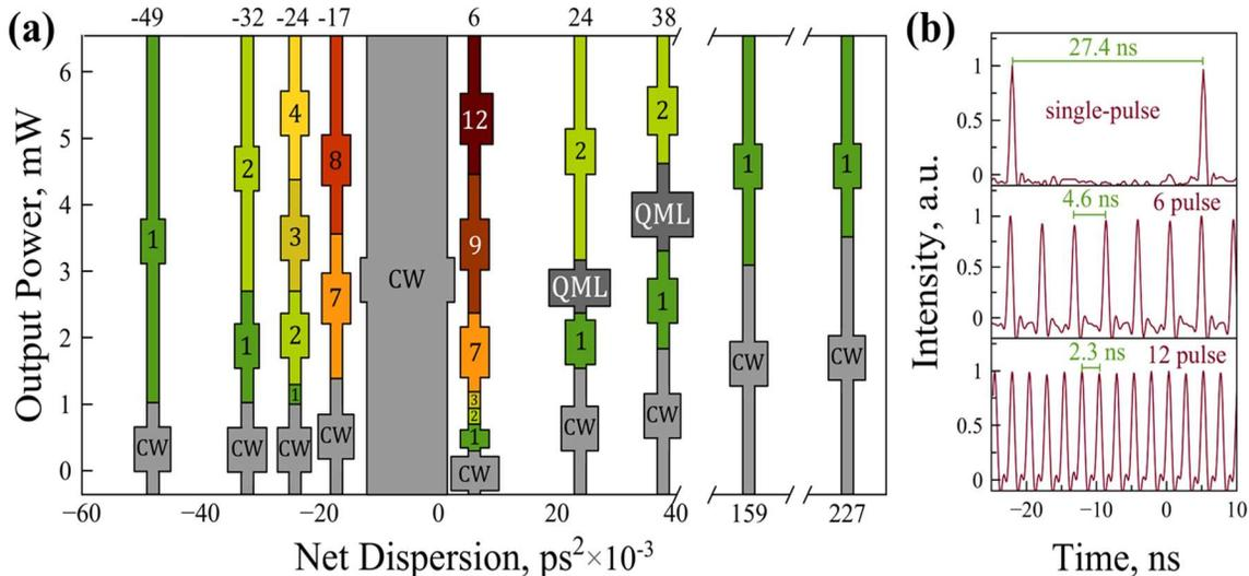
**Fig. 2.** a) Map of obtained laser generation regimes for various net dispersions and output powers. Numbers correspond to the order of harmonic mode-locking, CW denotes continuous wave generation and QML states for Q-switched mode locked transition regime. b) Harmonic mode-lock pulse trains of the 1st, 6th and 12th orders at near-zero net dispersion.
