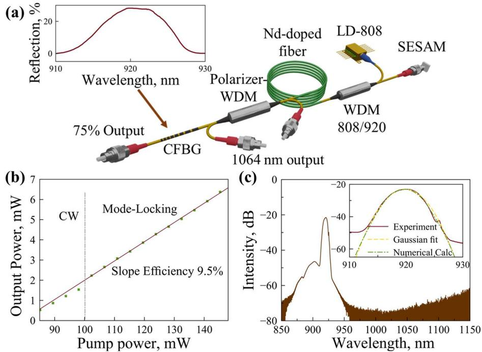
**Fig. 1.** a) Linear cavity mode-locked fiber laser scheme: CFBG – chirped fiber Bragg grating, WDM - wavelength division multiplexer, LD - laser diode, SESAM - semiconductor saturable absorber mirror, b) laser mode-locking threshold and slope efficiency, c) laser output pulse spectrum at 920 nm at the highest output power, limited by SESAM damage threshold of 10 mW. No sign of ASE at 1064 nm. Inset – experimental and numerical pulse spectra with Gaussian fit at anomalous net dispersion.
