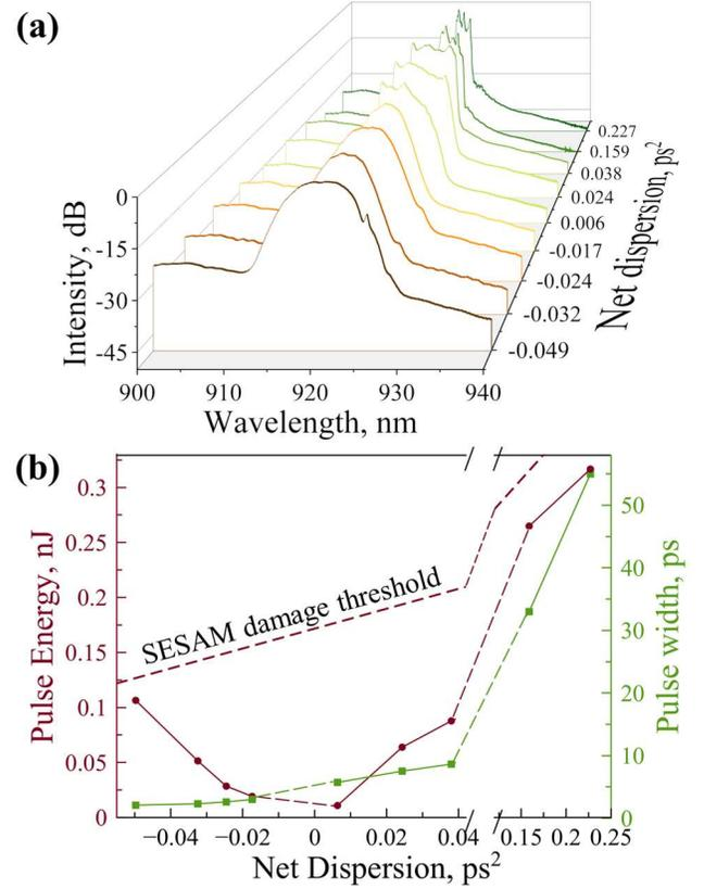
**Fig. 3.** a) Output pulse spectra for different net cavity dispersion. b) Pulse energy (brown) and pulse width (green) at different net dispersion. Brown dashed line shows SESAM damage threshold corresponding to the fixed average power calculated from saturation fluence inclined due to change of the cavity length. Lines connecting the point are presented for the eyeguiding.
