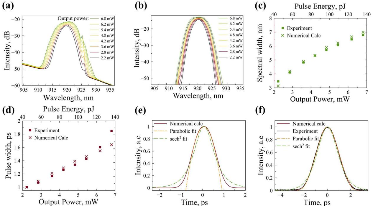
**Fig. 5.** a) Experimental and b) calculated pulse spectrum for different pump powers at anomalous net dispersion. Comparison of the experimental and calculated spectral c) and temporal d) widths of the pulse e) Simulated pulse shape on the output of the laser and its  $sech^2$  and parabolic fit. f) Experimental and simulated autocorrelation traces of the pulse and its  $sech^2$  and parabolic fits.
