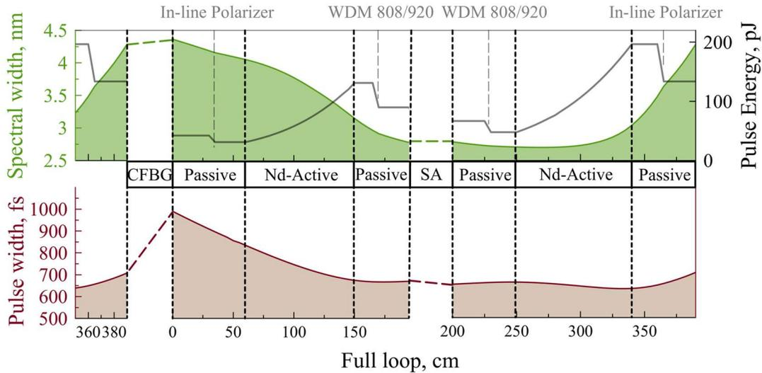
**Fig. 4.** Pulse energy, spectral and temporal widths dynamics inside the laser cavity.
