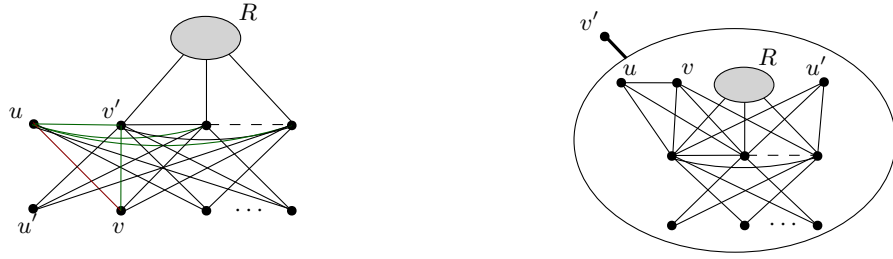
Fig. 9. The graph G with fill edges (green edges) including uv edge (red edge) where C_u = \{u\} and |K| \geq 4 , and its representation tree after addition of fill edges.
