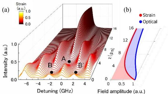
Figure 4: (a) Decomposition of the PLE spectrum at  $V_d$  of  $19.2 V_{rms}$  with respect to the depth of the YSO crystal. Color corresponds to the normalized strain. A, B, and B' indicate the points where the intensity becomes zero due to the destructive interference of the excitation. (b) Strain and optical field distribution along the  $z$ -axis.
