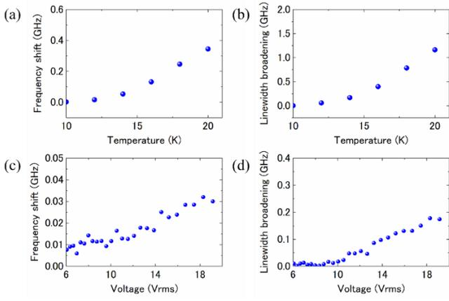
Fig. S5: Temperature dependences of the frequency shift (a) and linewidth broadening (b) of the optical resonance measured in an Er-doped YSO crystal without drive voltages. (c-d) Those caused by SAWs, which correspond to  $\Delta\omega/2\pi$  and  $\Delta\Gamma/2\pi$  in Eqs. 2d and 2e.
