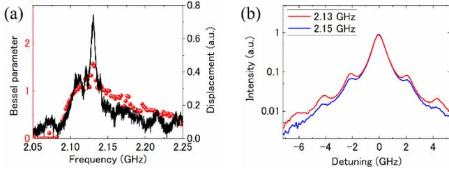
Fig. S3: (a) Drive frequency dependence of the Bessel parameter for pulse driving with  $V_d = 4.2 V_{rms}$  (red plots). The solid line shows the frequency response of the mechanical displacement measured by continuous driving with  $V_d = 12 V_{rms}$  with a Sagnac interferometer. (b) PLE spectra taken with drive frequencies of 2.13 and 2.15 GHz and  $V_d$  of 12  $V_{rms}$ .
