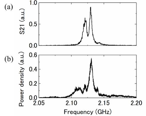
Fig. S2: (a) Electrically measured transmission spectrum ( $S_{21}$ ) between two IDT electrodes. (b) Spectral power density of SAW measured by optical interferometry.
