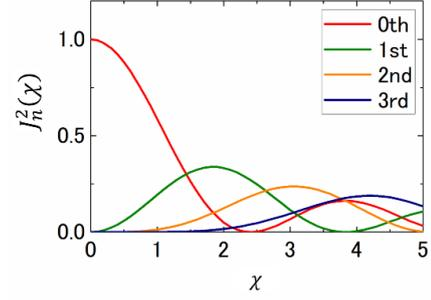
Fig. S4: Relation between the Bessel parameter,  $\chi$ , and the square of the amplitude of the  $n$ -th order Bessel function.
