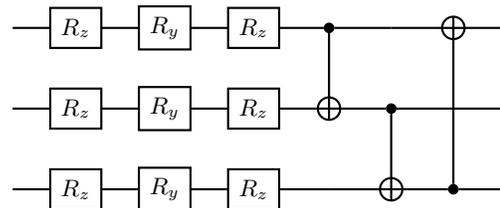
FIG. 5. A single layer of the Strong Entangling Layers ansatz for three qubits: it first applies single-qubit gates  $R_y$ ,  $R_z$  and  $R_y$  on all qubits which is then followed by nearest neighbour CNOT gates.
