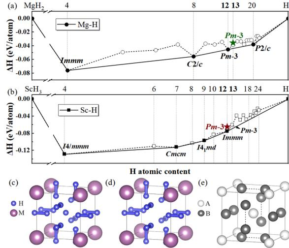
Fig. 1. The thermodynamic convex hull diagram of (a) Mg-H and (b) Sc-H systems at 300 GPa with ZPE included. The red and green stars near the convex hull correspond to the  $Pm\bar{3}$ - $\text{ScH}_{12}$  and  $Pm\bar{3}$ - $\text{MgH}_{13}$  phases, respectively. Crystal structure of (c)  $\text{MH}_{13}$ , (d)  $\text{MH}_{12}$ , and (e) the  $A15$  type structure ( $\text{AB}_3$ ,  $Pm\bar{3}n$ ).
