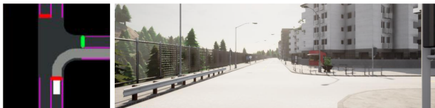
(a) Roach RL [34]: using semantic BeV as input during training time
