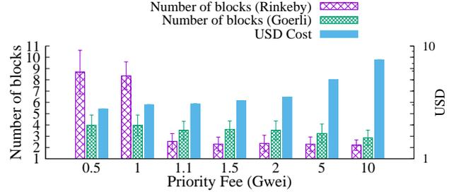
Figure 4: SUBMITRESPONSE Verification Time vs Priority Fee. Here, the base fee is 5 GWei.
