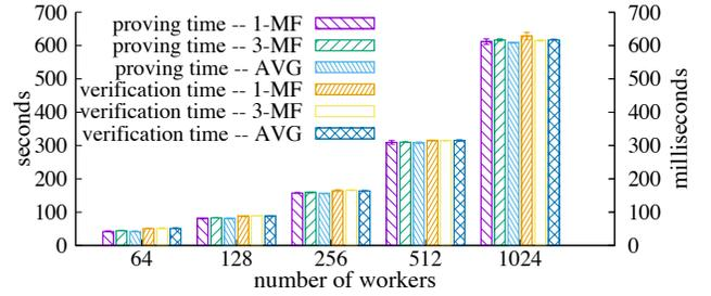
Figure 5: AUTHCALC: Proving & Verification Time vs. number of workers with 4 choices.
