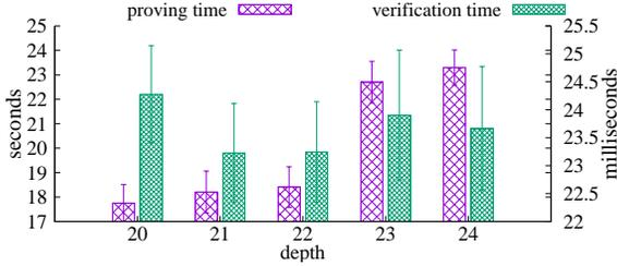
Figure 7: PROVEQUAL: Proving & Verification Time vs.  $MT$  Depth.
