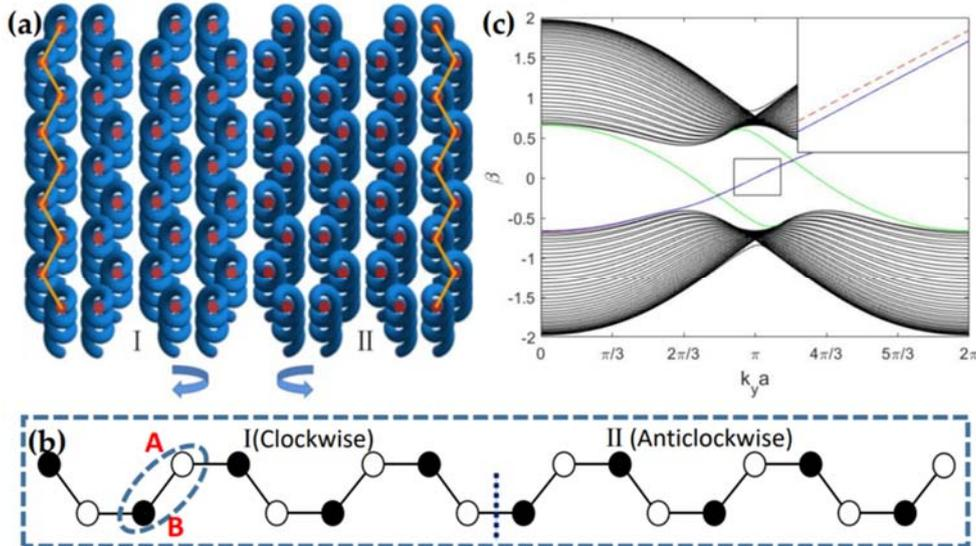
**Fig. 1.** (a) 3D lattice structure with opposite helicities. (b) Supercell of photonic Floquet lattices in (a) at  $\Delta\phi = 0$ . (c) Dispersion curves of edge states with  $R = 0.3d$  in (a). Inset is a magnified view of curve in the interval  $[8\pi/9, 10\pi/9]$  to illustrate the existence of two anti-chiral edge states.
