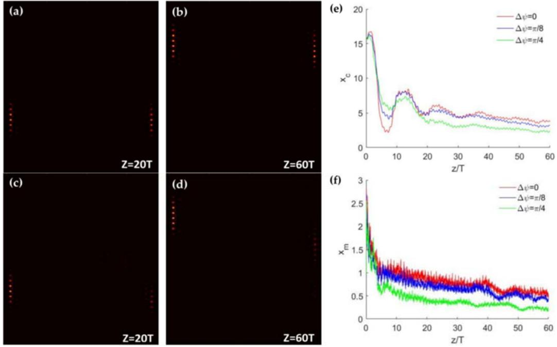
**Fig. 4.** (a) and (b) Transmission diagram when phase difference in the  $x$  direction is  $\pi/8$ . (c) and (d) Transmission diagram when phase difference in the  $x$  direction is  $\pi/4$ . (e) Beam center (centroid) in the  $x$  direction of  $\phi_2$  as function of relative propagation distance  $z/T$ . (f) Position of peak beam power  $x_m$  in the direction of  $\phi_2$  as function of relative propagation distance  $z/T$ .
