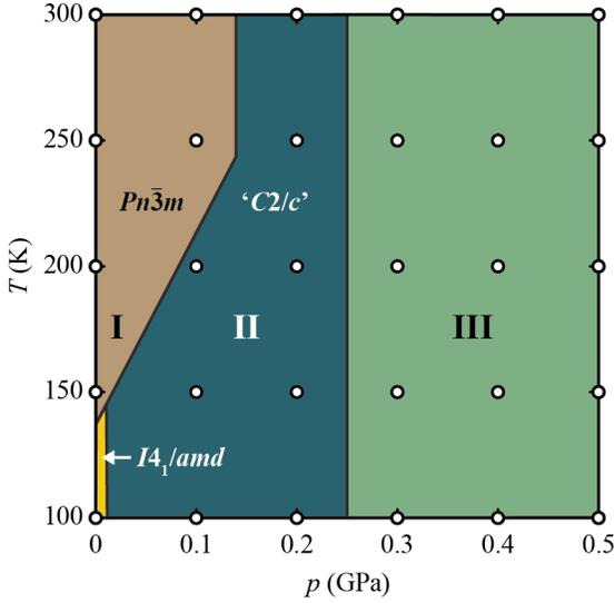
FIG. 4: Pressure/temperature phase diagram of  $\text{Cd}(\text{CN})_2$  as determined using neutron diffraction measurements. The grid of  $(p, T)$  values interrogated using HRPD are shown as open white circles. This diagram includes the low-temperature ambient-pressure  $I4_1/amd$  phase reported in Ref. 17.
