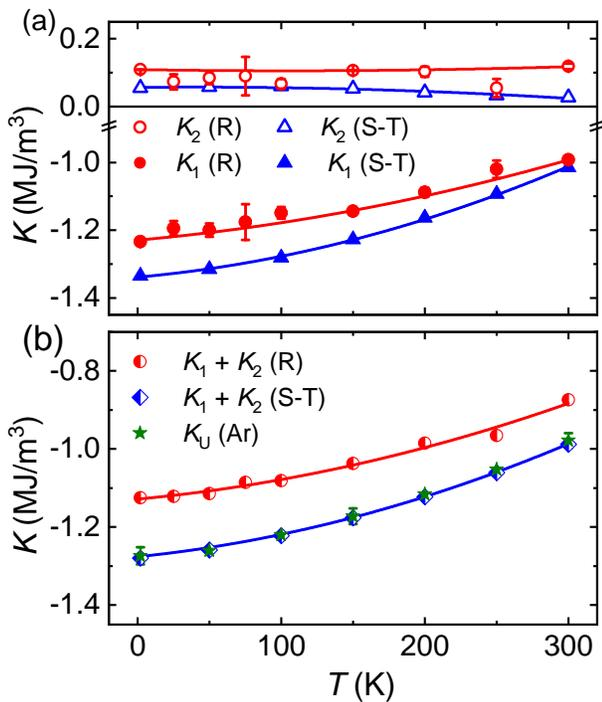
FIG. 4. (a) Temperature-dependent anisotropy constants  $K_1$  and  $K_2$  as determined from the angular dependence of the magnetisation (circles, marked as R) and by the S-T method (triangles). (b) The uniaxial constant  $K_u$  determined by the “area method” (Ar) is plotted together with  $K_1 + K_2$  taken from panel (a). Lines are guides to the eye.
