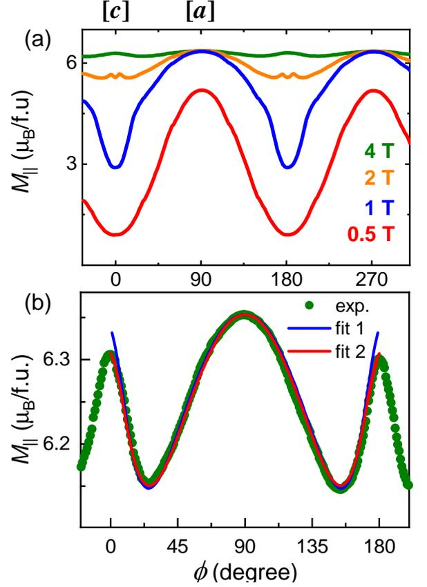
FIG. 3. (a) Angular dependence of the magnetisation measured in different fields at 300 K. The magnetisation component parallel to the field is detected. (b) Experimental data (open circles) and fit to the experimental data (solid lines) in 4 T at 300 K.
