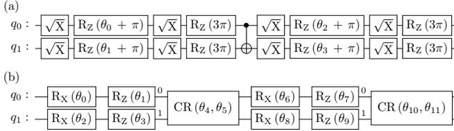
FIG. 3.  **$H_2$  Ansatz.** In the CNOT-based variational form (a) there are four parameters in virtual-Z gates. In the pulse-based variational form (b) there are twelve parameters.
