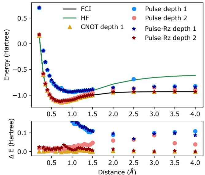
FIG. 13. **Simulated  $H_2$  dissociation curves.** The total energy is plotted against the distance between the two H atoms. The yellow triangles correspond to the CNOT-based Ansatz. The circles and stars correspond to the pulse-based wave function without and with the  $R_Z$  rotations, respectively. The black and green lines represent the full CI and Hartree-Fock energies, respectively. The bottom panel shows the absolute energy difference between the VQE simulations and the full CI energy.
