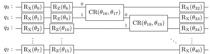
FIG. 9. **H<sub>4</sub> Pulse-based Ansatz.** The Ansatz has a total of 40 parameters. We first optimize the pulse amplitudes and durations, i.e. 32 parameters, and then the remaining 8 phases in the R<sub>Z</sub>( $\theta_i$ ) gates.
