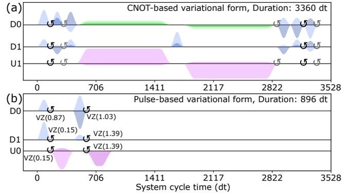
FIG. 5. **Optimized pulse schedules for  $H_2$  at  $0.2 \text{ \AA}$ .** (a) CNOT-based and (b) pulse-based Ansätze. The circular arrows indicate zero-duration virtual-Z gates (VZ). In the CNOT-based Ansatz the black virtual-Z gates are the only parameterized instructions. The drive channels  $D_i$  indicate single-qubit pulses on qubit  $i$  and the control channels  $U_j$  indicate cross-resonance tones, see details in Appendix E.
