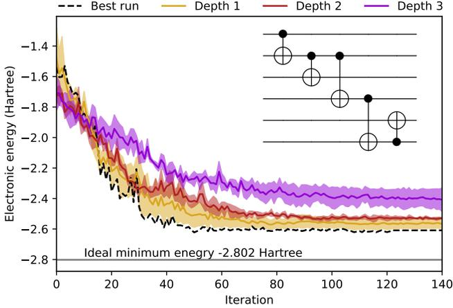
FIG. 15. **VQE on  $H_3$  with different depths.** The inset shows the structure of the entangler that was repeated  $p$  times with  $p + 1$  layers of parameterized  $R_Y(\theta)$  gates. The bond distance is 1.43 Å and the angle is 40°. The solid lines and shaded areas show the mean and standard deviation, respectively, of three runs. The dashed black line shows the best run which was a depth-one run.
