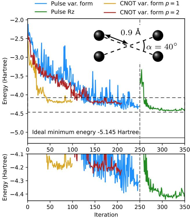
FIG. 10. **Electronic energy of  $H_4$ .** The gray horizontal line shows the minimum energy. The depth of the Ansatz is  $p$ . The bottom panel corresponds to the region between the dashed horizontal lines. The vertical gray line shows the point where we freeze the amplitudes and duration and optimize the phase.
