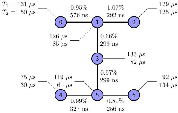
FIG. 16. **Coupling map of *ibm\_lagos*.** The numbers attached to each qubit represent the  $T_1$  and  $T_2$  times as reported by the backend. The top and bottom numbers of each edge indicate the error of the CNOT gate and its duration, respectively.
