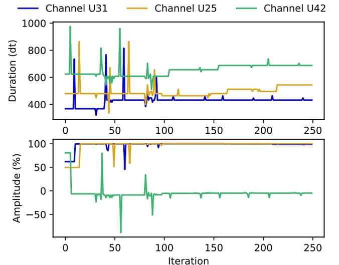
FIG. 12. **Parameter optimization.** The pulse parameters of the cross-resonance pulses played on the channels U25, U31, and U42, shown in Fig. 11, during the COBYLA optimization of  $H_4$ . The minimum duration of the GaussianSquare pulses is 256 samples due to the Gaussian flanks.
