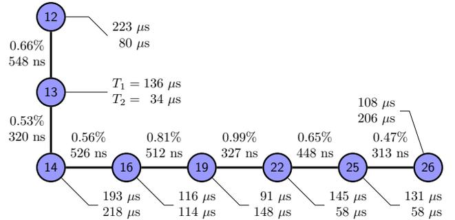
FIG. 17. **Qubits of *ibmq\_mumbai* to run  $H_4$ .** The numbers attached to each qubit represent the  $T_1$  and  $T_2$  times as reported by the backend. The top and bottom numbers of each edge indicate the error of the CNOT gate and its duration, respectively.
