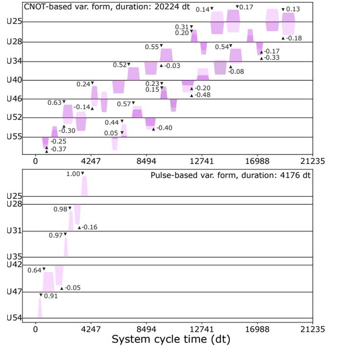
FIG. 11. **Optimized pulse schedules for  $H_4$ .** The top and bottom panels show the schedules of the depth-two CNOT and pulse-based Ansatz, respectively. For visualization purposes we only show the cross-resonance drives and omit the single-qubit pulses as well as the rotary tones in the CNOT gates.
