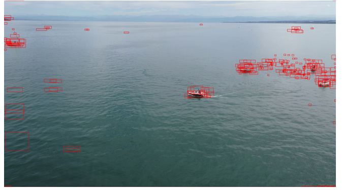
Fig. 6. Before NMS, there are many low-confidence detections, but they cluster around actual objects. Ignoring the confidence, these detections would yield a recall value of one. For visualization, only one-colored boxes.
