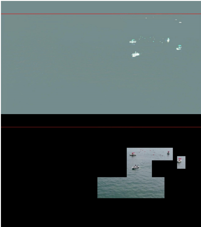
Fig. 11. Difference anomaly map aggregated in 3D space over several frames (top) and resulting regions of interested (bottom).
