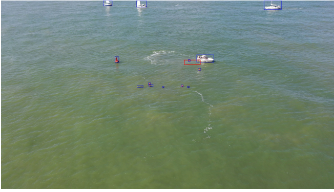
Fig. 5. Blue boxes are true positive detections, the red box is a false positive swimmer detection that was successfully filtered out by analyzing the distance-size relation.
