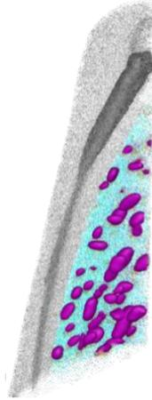
Supplementary Figure 3. APT reconstruction of a GB containing dataset. The coloured features display the location of the measurements shown in Table 2.
