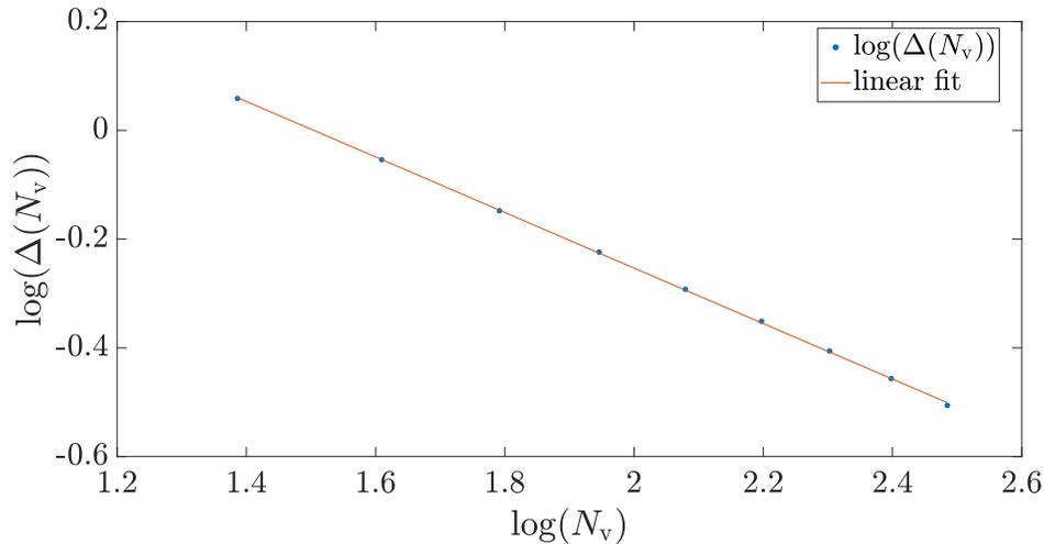
Figure 3: The plot shows the scaling of the energy gap  $\Delta$  in the dependence of the maximum number of vertices  $N_v$  of graphs used in the NLCE in a double-logarithmic plot. A linear fit of good quality shows that the behaviour is algebraic with an exponent of  $\kappa = -0.51$ .
