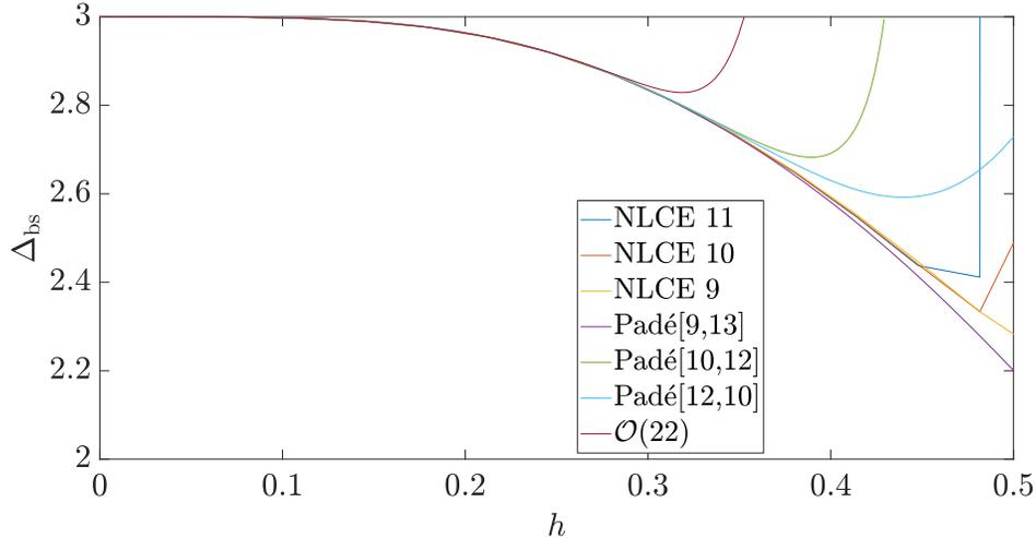
Figure 4: The figure shows an NLCE expansion of the bound-state gap  $\Delta_{\text{bs}}$  in dependence of the number of nodes of the graphs taken into account. The expansion converges only until around  $h \approx 0.35$ . The convergence problems are caused by avoided level crossings occurring on finite graphs. As more graphs are taken into account in the expansion convergence becomes gradually worse. Padé extrapolations and bare series results are also shown.
