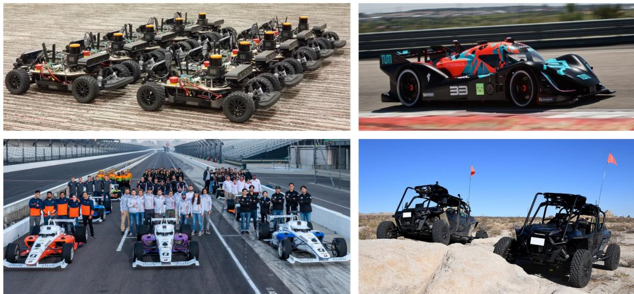
Figure 1: Examples of real-world autonomous racing competitions. (Top-Left) F1 Tenth, using a 1:10 scaled vehicle. (Top-Right) Roborace, using a full-scale electric race car. (Bottom-Left) Indy Autonomous Challenge (IAC), using a Dallara AV-21 retrofitted Indy Lights class chassis. (Bottom-Right) DARPA-RACER program, using autonomous ground combat vehicles in unstructured off-road terrain at speeds.
