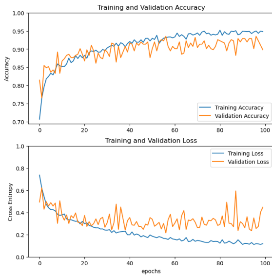
(a) Convergence pattern of training and validation accuracy and sparse categorical crossentropy loss function using proposed model up to epoch 100 in Sipakmed dataset
