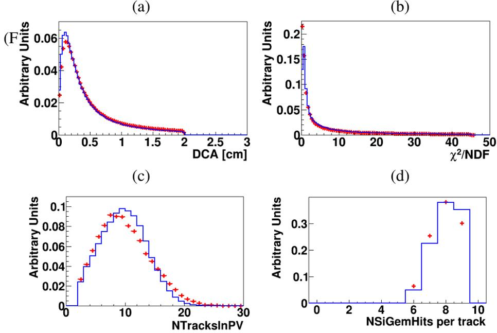
Figure 8: Comparison of experimental distributions (red crosses) and GEANT distributions of events generated with the DCM-SMM model (blue lines), in Ar+A collisions at 3.2 AGeV: (a) DCA, distance of closest approach to the primary vertex; (b)  $\chi^2/\text{NDF}$  of reconstructed tracks; (c) number of reconstructed tracks in the primary vertex in Ar+Cu interactions; (d) Hits per track in the 3 forward Si and 6 GEM detectors.
