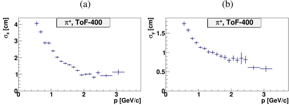
Figure 4:  $\sigma_x$  (a) and  $\sigma_y$  (b) of the Gaussian fit of the ToF-400 hit residuals with respect to positively charged pions depending on the particle momentum.
