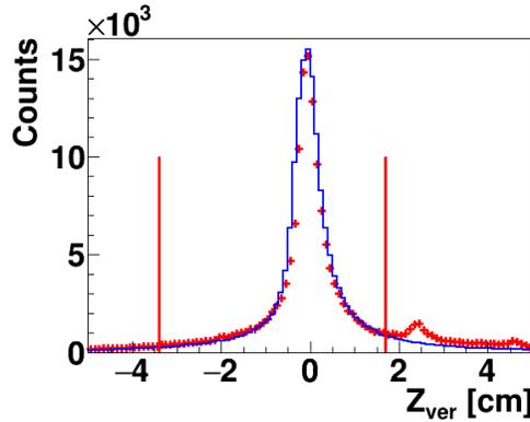
Figure 3: Distribution of the primary vertices along the Z axis for data (red crosses) and simulated events (blue histogram). The vertical lines limit the Z region accepted for the data analysis.
