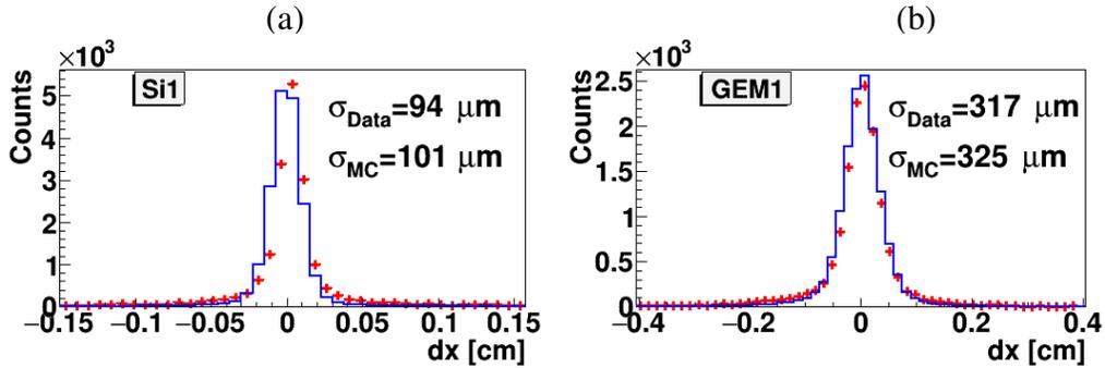
Figure 7: Residual distributions of hits in the X projection (magnet deflection plane) with respect to reconstructed tracks: (a) - in the first forward silicon plane, (b) - in the first GEM plane. The experimental data are shown as red crosses, and the simulated data are shown as blue histograms.
