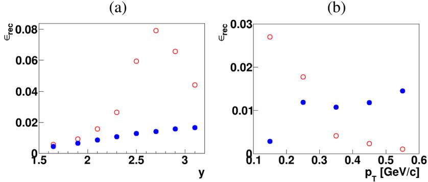
Figure 9: Reconstruction efficiency of  $\pi^+$  produced in Ar+Sn collisions, detected in ToF-400 (open red circles) and ToF-700 (full blue circles) as function of rapidity  $y$  (a) and  $p_T$  (b). The efficiency includes both acceptance and reconstruction.
