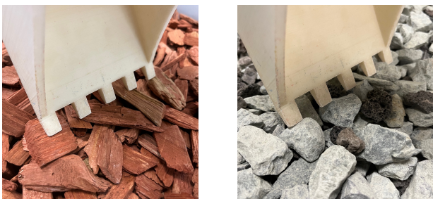
Fig. 3. Vertically downward bucket movements will result in large contact forces and jamming. The bucket cannot penetrate into the terrain. An optimal strategy should sweep the surface of the terrain for downstream penetration.
