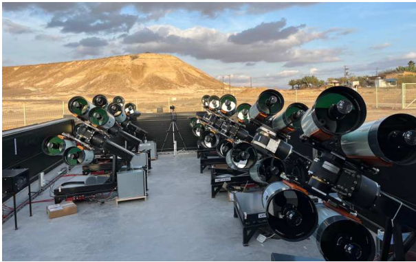
FIG. 2.— LAST with 32 telescopes installed. The enclosure is fully open.
