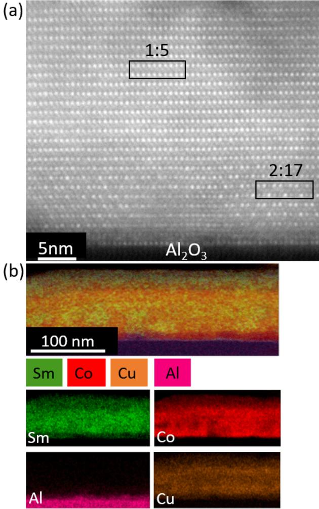
Figure 6: (a) High resolution HAADF STEM image showing the interface of the SmCo<sub>4</sub>Cu thin film to the Al<sub>2</sub>O<sub>3</sub> substrate. The dumbbell pattern of atomic columns reveals the presence of the Sm<sub>2</sub>Co<sub>17</sub> phase. (b) Chemical composition mapping of Sm, Co and Cu extracted from STEM/EDX spectrum imaging. Note the distribution of Co and Cu is not uniform.
