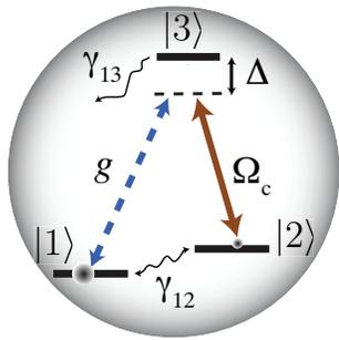
FIG. 3. Energy-level diagram for a  $\Lambda$ -type atom driven by control and probe fields. For simplicity, the detuning is set to be the same for both transitions (i.e. zero two-photon detuning).  $\Delta$  is one-photon detuning,  $\gamma_{ij}$  is damping rate between levels  $i$  and  $j$ .
