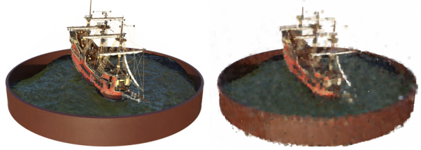
Figure 5. Comparison with dense grid field representation. Tetra-NeRF on the left , dense grid on the right . We used a comparable number of parameters for both methods (the dense grid having slightly more parameters). Due to the adaptive nature of tetrahedra fields, Tetra-NeRF produces significantly better rendering as it is able to focus on relevant parts of the scene.
