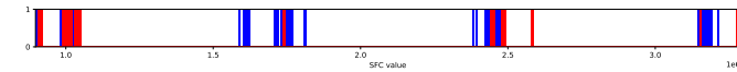
(c) Zebra-pattern representing the single-dimensional Morton codes corresponding to the acceleration tuples from Fig. (b) on a Z-order curve.
