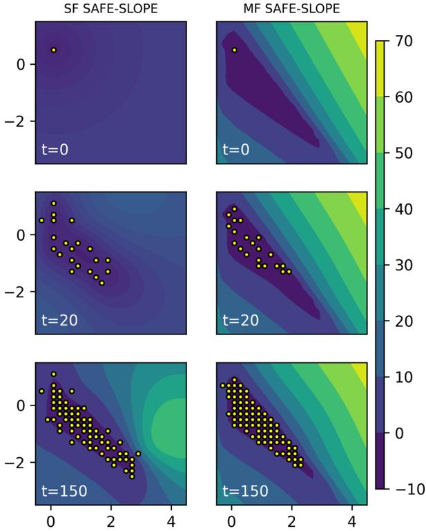
Fig. 2. Progression of sampling using SAFE-SLOPE on single- and multi-fidelity models. Darker regions indicate areas of lower LQR costs. By utilizing an AR-1 model, fewer unstable points are tested.
