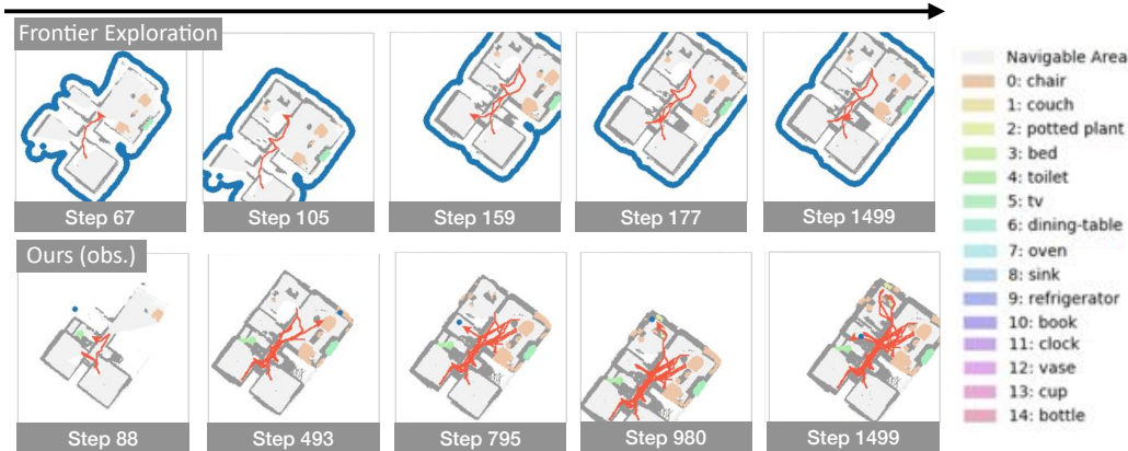
Figure 5: Rollouts by Frontier-Based Exploration vs. Modular policy (obs cov): FBE properly covers the scene, but does not collect a large diversity of viewpoints, while the modular policy enters the rooms and thus provides richer training data for the neural field.
