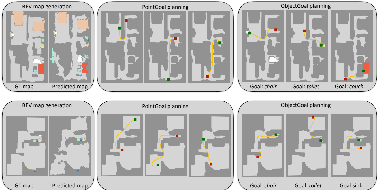
Figure 10: BEV map tasks: Generation of semantic BEV maps (Left), PointGoal (Middle) and ObjectGoal planning (Right). NeRF training data is collected by Ours (obs) .
