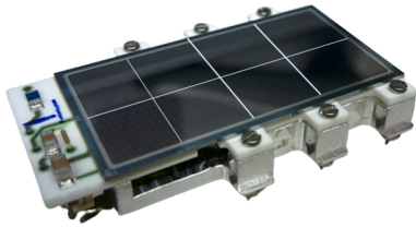
Figure 2. Silicon drift detector array for the SIDDHARTA-2 experiment with eight read-out cells indicated by the grey lines. The array is mounted on a ceramic carrier.
