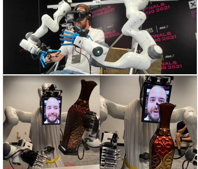
Fig. 1. Operator interacting through the NimbRo Avatar system with a human recipient at the ANA Avatar XPRIZE semifinals. Top: Operator at remote site. Bottom: Two different facial expressions of the operator animated with our method. See also the supplementary video for an animated version.
