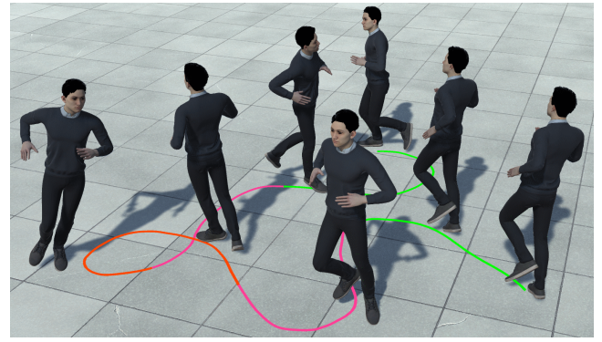
Fig. 8: Our TPTN can synthesize motions heading along a complex trajectory transitioning from jumping-R to jumping-L, to running, then to jumping-L, and ending with jumping-R (from 1m21s to 1m32s in the accompanying video).
