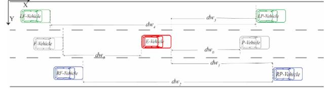
Fig.3 The headway distance between the E-vehicle and surrounding vehicles
