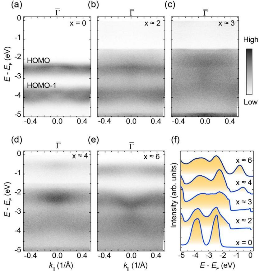
FIG. 2. (a) Band structure of 3ML pristine  $C_{60}$  film grown on bilayer graphene/SiC substrate. (b-e) Evolution of the band structure of  $K_xC_{60}$  film with K doping. (f) Integrated EDCs of  $K_xC_{60}$  films in (a-e). Data were collected using helium lamp ( $h\nu = 21.2$  eV) at 13 K.
