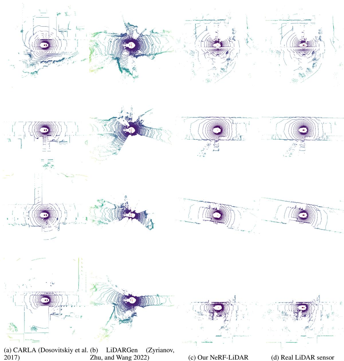
Figure 10: Comparisons of results between our NeRF-LiDAR and other existing LiDAR simulation methods. (a) Method (Dosovitskiy et al. 2017) that creates virtual world for LiDAR simulation. (b) Diffusion model used for LiDAR generation (Zyrianov, Zhu, and Wang 2022). (c) Our NeRF-LiDAR can generate realistic point clouds that is nearly the same as the real LiDAR point clouds (d). Real LiDAR sensor *Zoom in to see details*
