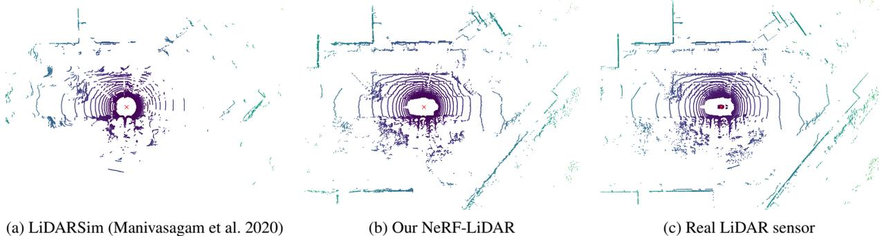
Figure 6: Comparison between our NeRF-LiDAR and LiDARSim (Manivasagam et al. 2020). Sparse aggregated point cloud leads to poor-quality mesh when reconstructing scenes. Thus, the simulated LiDAR points lose reality compared to NeRF-LiDAR.
