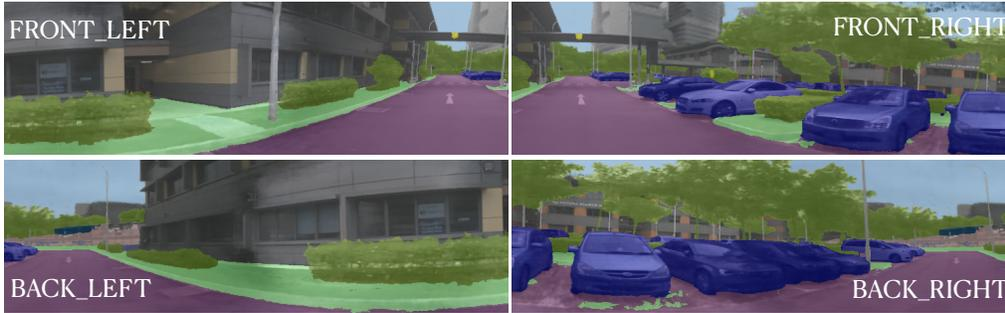
Figure 8: NeRF-LiDAR can also render high-quality RGB novel views along the the LiDAR. We simulate a 4 cameras and one LiDAR sensor configuration that is different from the neScenes configuration in the training dataset.
