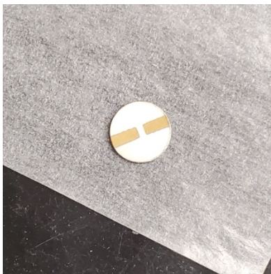
Figure S3. Image of LLTO pellet with Au sputtered contacts.
