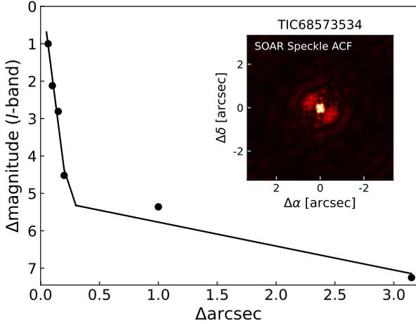
**Fig. B.1.** Sensitivity curve and auto-correlation function from the speckle imaging with SOAR in *I*-band, which is similar to the TESS passband.
