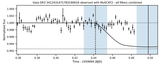
**Fig. B.4.** Light curve of Gaia DR3 3412431471783190016 covering the expected transit ingress observed with MuSCAT2. The dots with uncertainties show the MuSCAT2 observations, the solid line visualises the transit, the solid vertical line shows the expected transit center, and the slashed vertical line shows the expected beginning of the transit. The observations clearly show that the transit signal does not arise from Gaia DR3 3412431471783190016.
