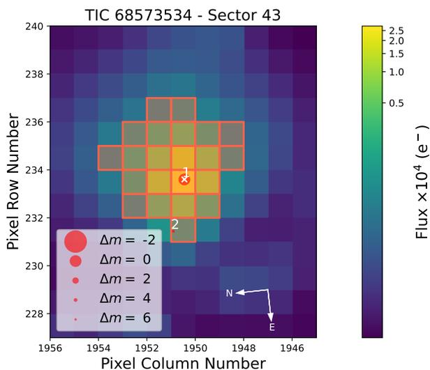
**Fig. 2.** Results of `tpfplotter` showing HD 31221, the aperture used for the photometry and the only star that is known to be located in the aperture within  $\Delta m = 6$  magnitudes. The TESS pixel scale is  $21''$ .
