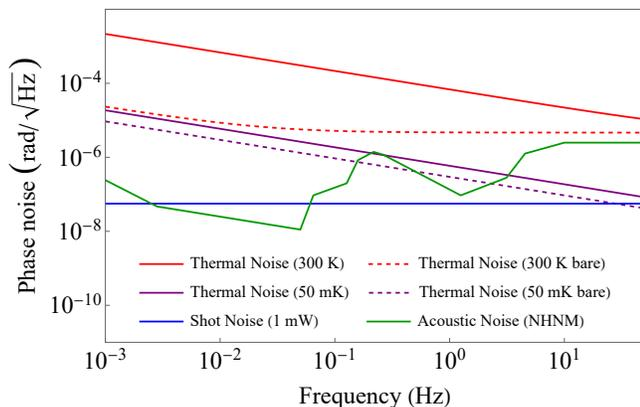
FIG. 2. **Estimated phase noise for the fiber-based detector:** Contributions are included from each of the noise sources detailed in Section IV. Several thermal noise curves are included, corresponding to fibers with (solid lines) and without (dashed lines) polymer coatings at temperatures of 300 K and 50 mK.
