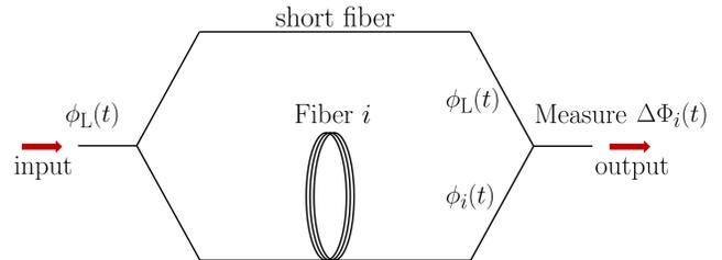
FIG. 5. **Illustration of fiber interferometer, with relevant phases marked:** The inferred output phase difference  $\Delta\Phi_i(t) = \phi_L(t) - \phi_i(t) + \delta\phi_i^{\text{shot}}$  is determined by measuring the output optical power.
