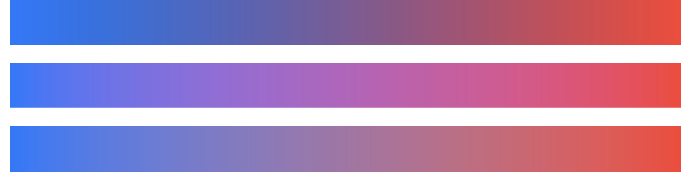
Figure E.11: Linear interpolation between blue and red in device color space (sRGB), linear sRGB space, and perceptually uniform color space (okLab). First transition has noticeable brightness change, the second one has unexpected strong hue change in purple direction, while the last one appears to be OK.
