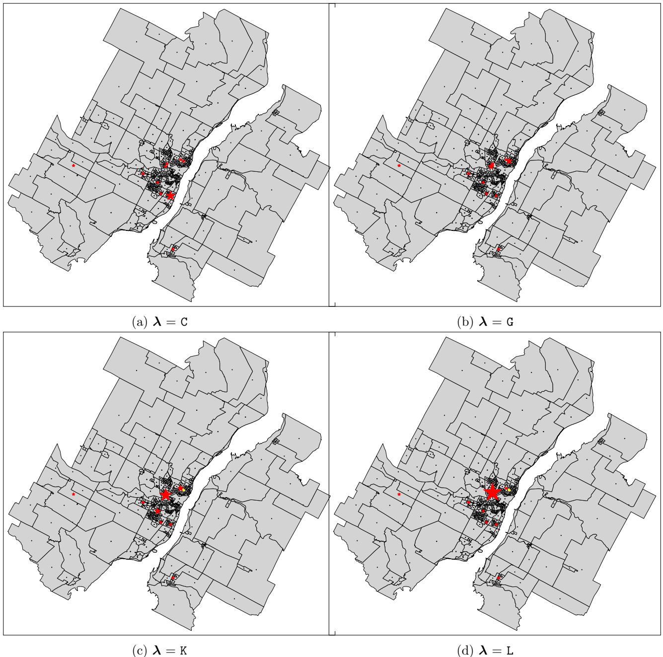
FIGURE 4. Real-Data with |\mathcal{I}| = 317 , |\mathcal{J}| = 4 , |\mathcal{T}| = 4 , |\mathcal{S}| = 5 , and T = 4.5 . Example of the optimal placement of charging stations for electric vehicles in the city of Trois-Rivières, Québec, for different \lambda -values. Red stars denote open stations, with the size of the star indicating the number of outlets, yellow stars represent closed stations, and black points indicate the client class for each region.
