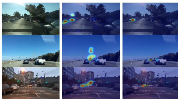
Fig. 1: Camera images from BDD-A (first column), Gaze map from BDD-A (second column), Cleansed gaze map from BDD-A (third column).
