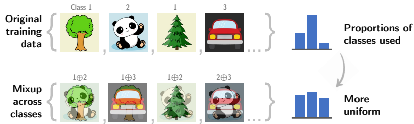
Figure 1: Selective mixup is a family of methods that replace the training data with combined pairs of examples fulfilling a predefined criterion, e.g. pairs of different classes. As an overlooked side effect, this modifies the training distribution: in this case, sampling classes more uniformly. This effect is responsible for much of the resulting improvements in OOD generalization.
